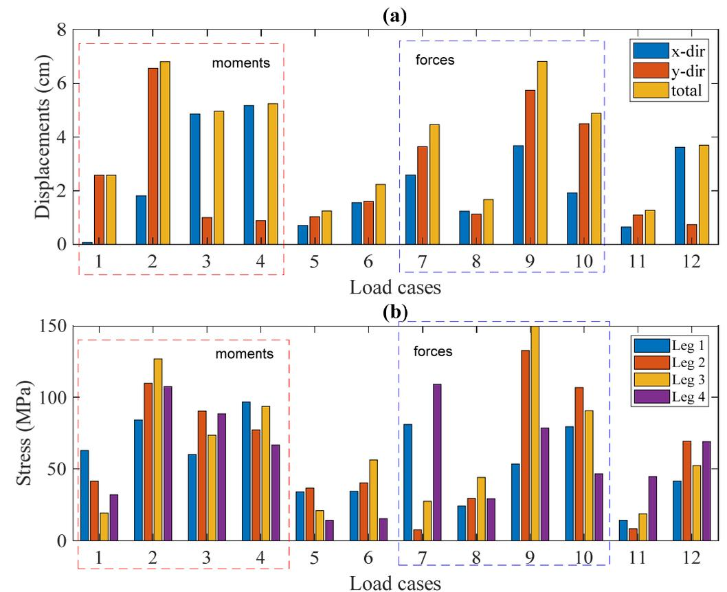
**Figure 8.** Structural responses under DLC loads: (a) displacements at IP (cm); (b) stresses at lower jacket legs (MPa).
