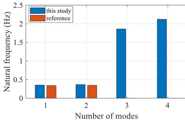
**Figure 5.** Comparison of natural frequencies of the support structure.
