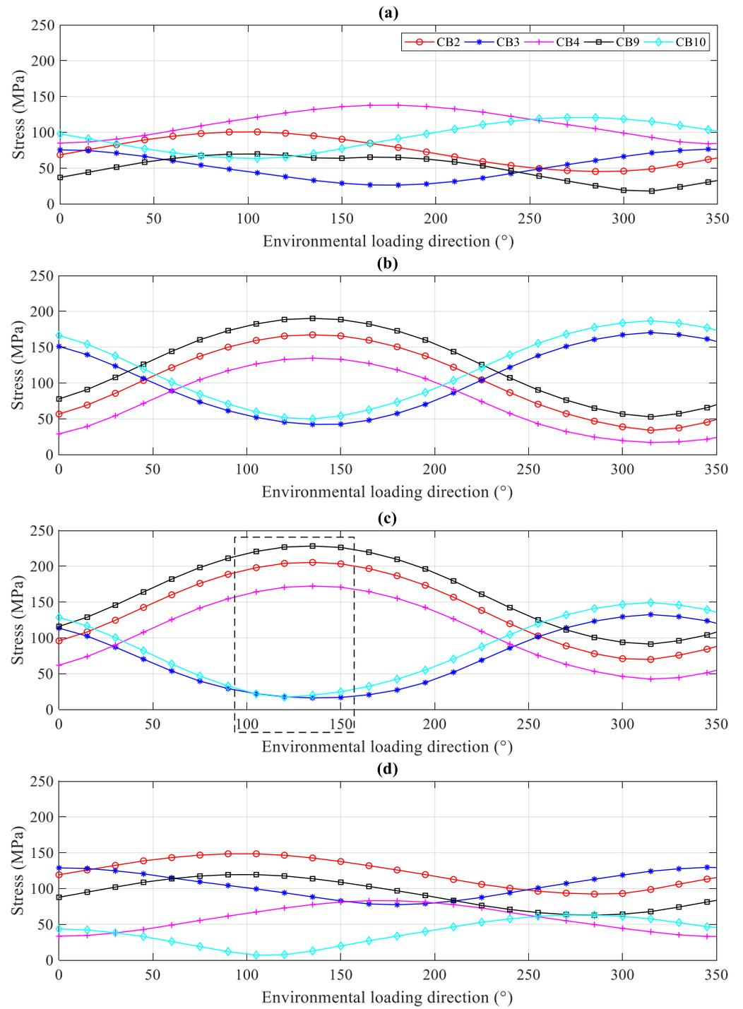
Figure 10. Stresses at lower jacket legs under combined loads: (a) Leg 1; (b) Leg 2; (c) Leg 3; (d) Leg 4.
