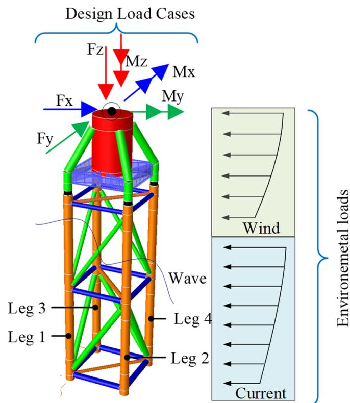
**Figure 6.** Loads acting on the 4-leg jacket substructure.
