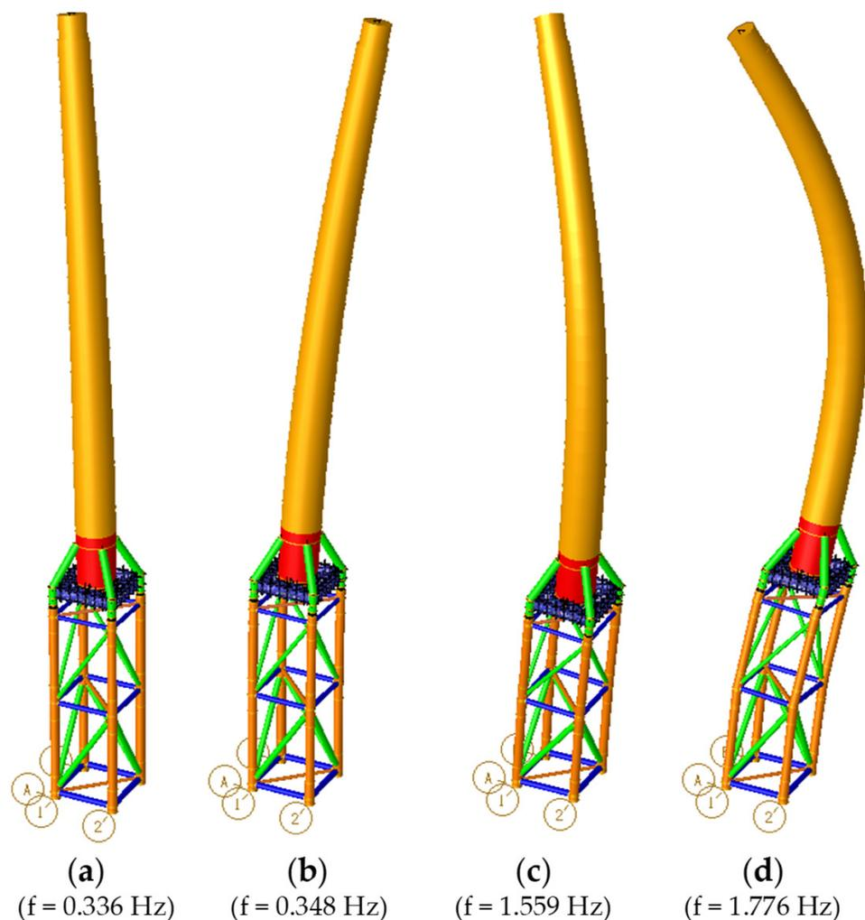
**Figure 4.** Mode shapes of the support structure: (a) Mode 1; (b) Mode 2; (c) Mode 3; (d) Mode 4.
