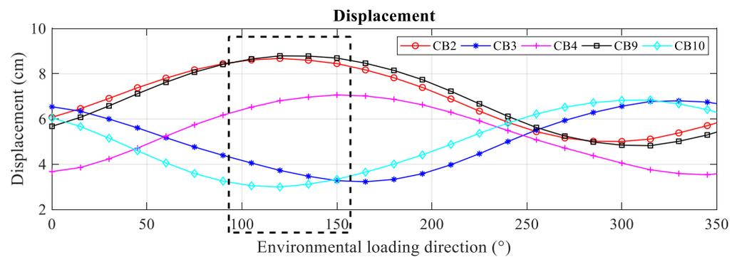
**Figure 9.** Lateral displacements at IP under combined loads.
