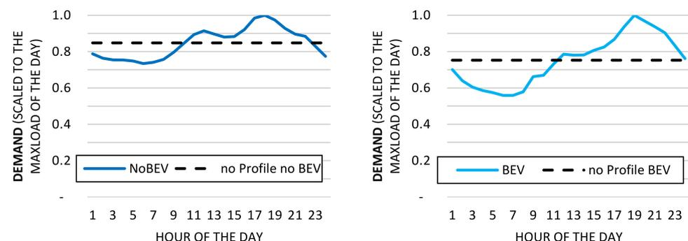
**Figure 11.** Exemplary depiction of the demand curves for the model runs without *BEV* (left graph) and with *BEV* demand (right graph) one time without profiles (black dashed lines) and with profiles (blue lines) for an exemplary day.
