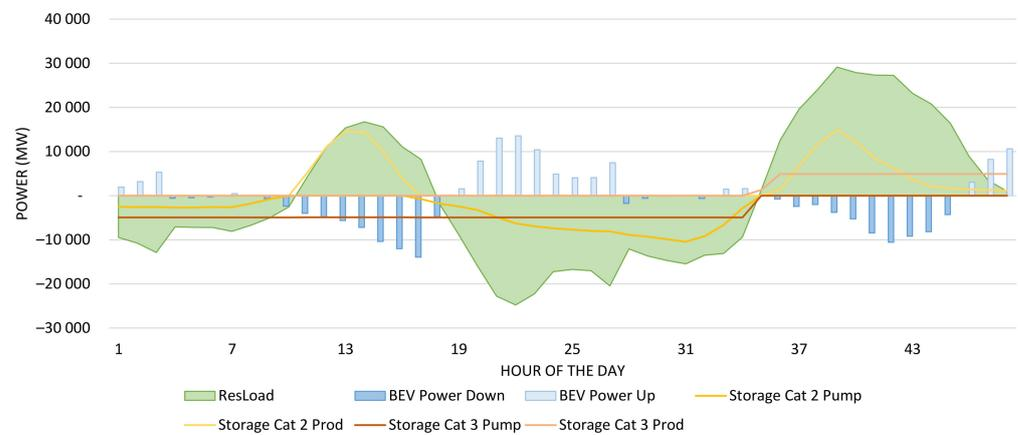
**Figure 8.** Interaction between the *DSI*-flexibility (blue/light blue) and the storages (Cat 2 in yellow/light yellow, Cat 3 in red/light red) to meet the given residual load (green area) for two exemplary days.
