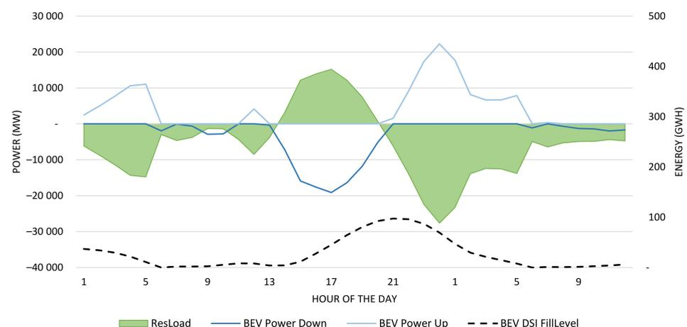
**Figure 6.** Use of BEV-DSI potential (PowerUp in light blue, PowerDown in blue) for 36 h to meet the residual load demands (ResLoad, green area). The corresponding fill level of the DSI storage is depicted in black dashes on the secondary axis.
