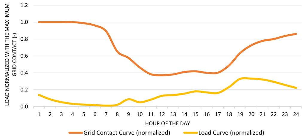
**Figure 2.** Depiction of the simulated realized charging profile for an exemplary day (yellow line), the maximum possible charging of all cars connected to the station (orange line), the maximum positive flexibility (blue arrow) and maximum negative flexibility (black arrow), normalized values.
