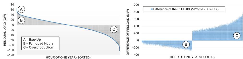
**Figure 12.** Residual load duration curve, congruent for the *BEV* scenarios (left graph), with the areas for the back-up need (A); full-load-hours (B) and overproduction (C). The right graph shows the resulting differences between the scenario without and with *BEV*-*DSI* concerning the FLH-reduction (B) and the overproduction (C). Concept of the figure based on [27].
