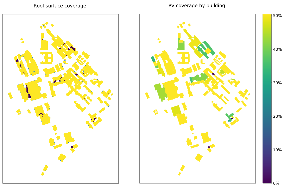
Figure 5. Roof surfaces selected for PV placement based on a minimum threshold of 800 \text{ kWh/m}^2/\text{yr} (left) and area of PV installed per unit area of roof surface for each building based on a minimum threshold of 800 \text{ kWh/m}^2/\text{yr} (right).
