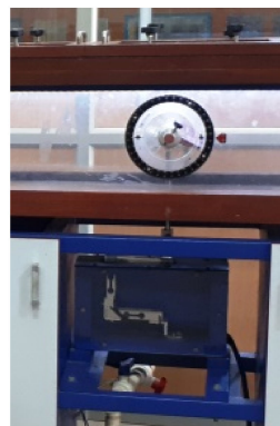
Figure 6. Test airfoil mounted to the three-component force balance setup.
