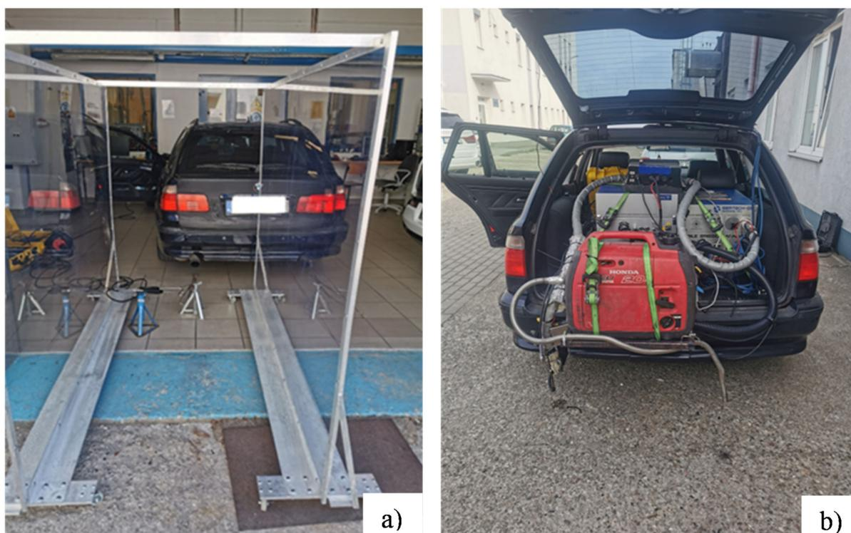
**Figure 4.** Test vehicle—measurement of the concentration of the exhaust cloud behind (a) a stationary vehicle; (b) a moving vehicle.
