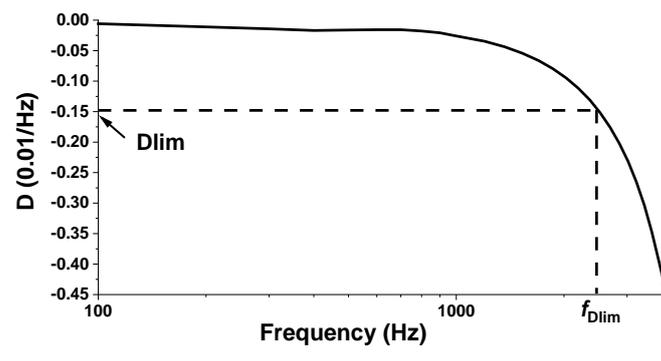
**Figure 4.** Behavior of the frequency derivative of the Voltage Transformer (VT) ratio error from the SFS test. The point  $[f_{Dlim}, D_{lim}]$  identifies the limit beyond which the linear effects affecting the ratio error are predominant.
