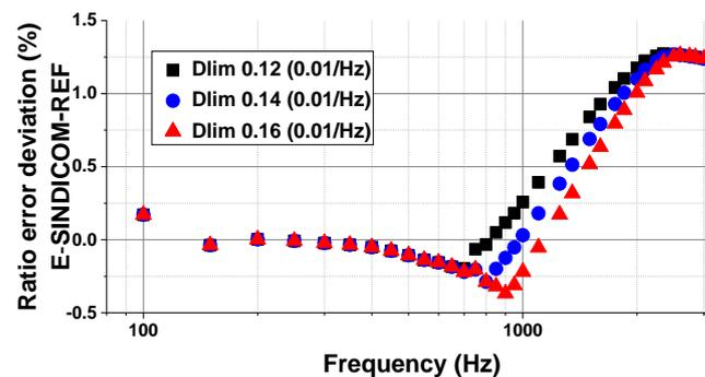
**Figure 7.** VT1 ratio error deviation vs frequency with different values for  $D_{lim}$  and  $f_{Dlim}$ .
