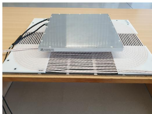
**Figure 2.** Illustrative implementation of two coils for a magnetic resonant WPT.
