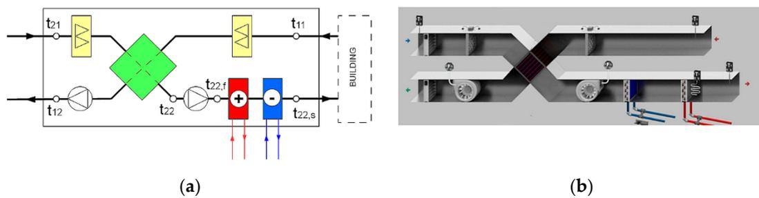
**Figure 2.** (a) Schematic view of specific temperatures in the air handling unit (AHU); (b) view of the AHU in the Building Management System (BMS).
