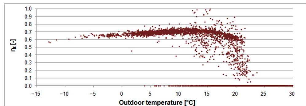
**Figure 12.** Heat recovery efficiency versus outdoor air temperature.
