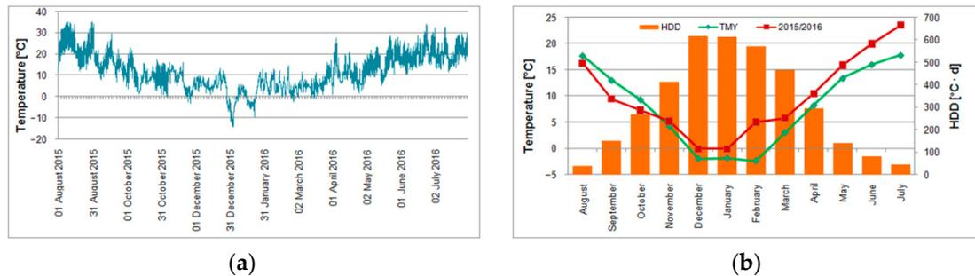
**Figure 3.** Meteorological conditions in Katowice: (a) outdoor air during measurements; (b) mean monthly outdoor air temperature and heating degree days.
