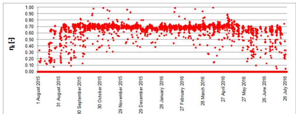
Figure 8. Hourly efficiency of heat recovery from 1 August 2015 to 31 July 2016.
