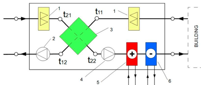
Figure 1. Schematic view of an air handling unit with a cross-flow heat exchanger.
