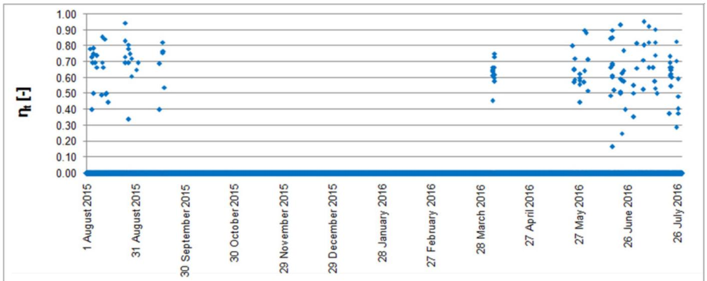
Figure 14. Hourly efficiency of cold recovery from 1 August 15 to 31 July 16.
