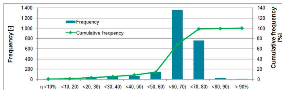
Figure 11. Histogram of calculated hourly efficiency of heat recovery.
