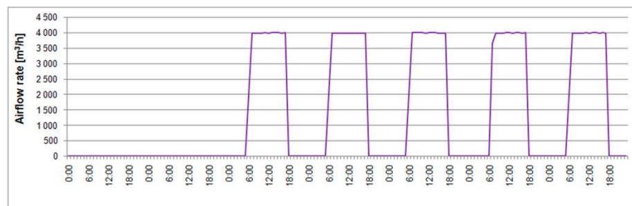
**Figure 6.** Supply airflow rate from 1 August 2015 to 7 August 2015.
