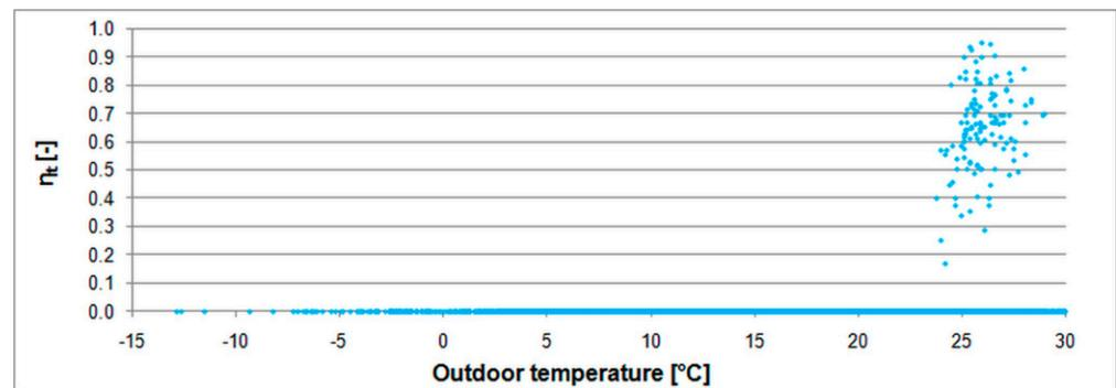
Figure 15. Cold recovery efficiency versus outdoor temperature.
