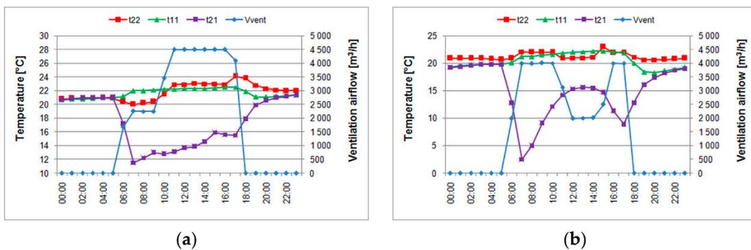
Figure 10. Temperatures  $t_{11}$ ,  $t_{21}$ , and  $t_{22}$  and ventilation airflow on (a) 12 April 2016; (b) 4 November 2015.
