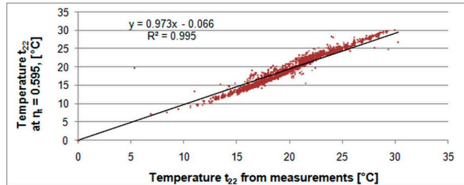
Figure 13. Correlation of temperature  $t_{22}$  calculated from measurements and for constant  $\eta_t$ .
