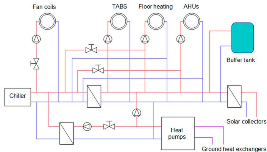
**Figure 5.** Schematic diagram of the heating, ventilation, and air conditioning system in the building.
