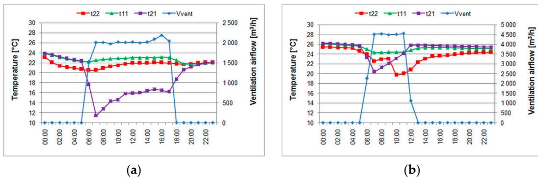
Figure 9. Temperatures  $t_{11}$ ,  $t_{21}$ , and  $t_{22}$  and ventilation airflow on (a) 21 September 2015; (b) 27 July 2016.
