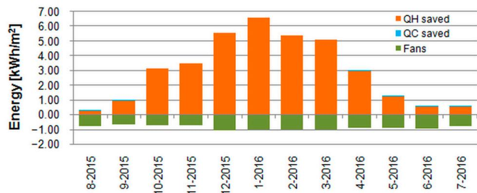
Figure 16. Unit electricity consumption (-), heat and cold savings (+).
