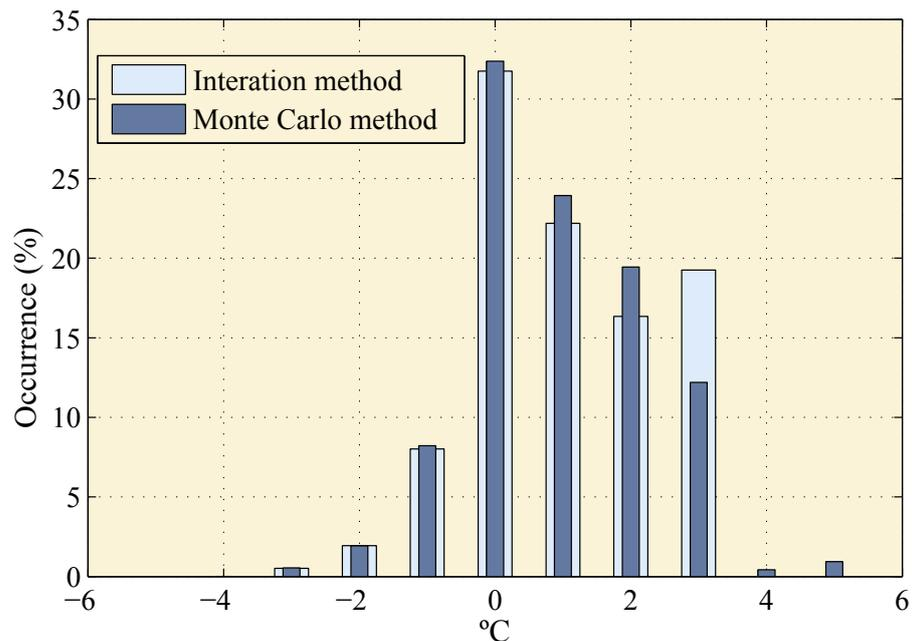
Figure 19. Differences between measured and estimated conductor temperature.
