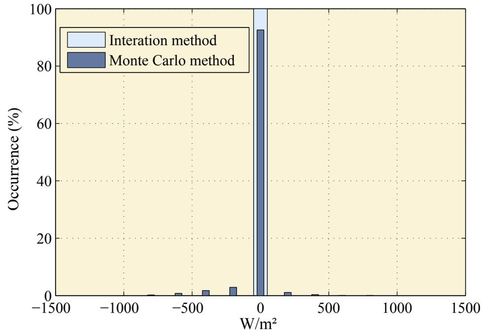
Figure 18. Differences between measured and effective solar radiation.
