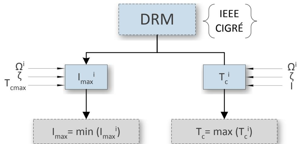
Figure 1. Dynamic Rating Management (DRM) system flowchart.
