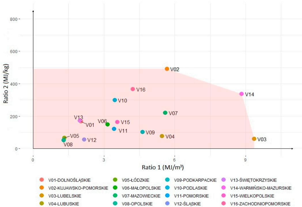
Figure 4. Efficiency of heat production from biogas and biomass in 2012 in Poland.
