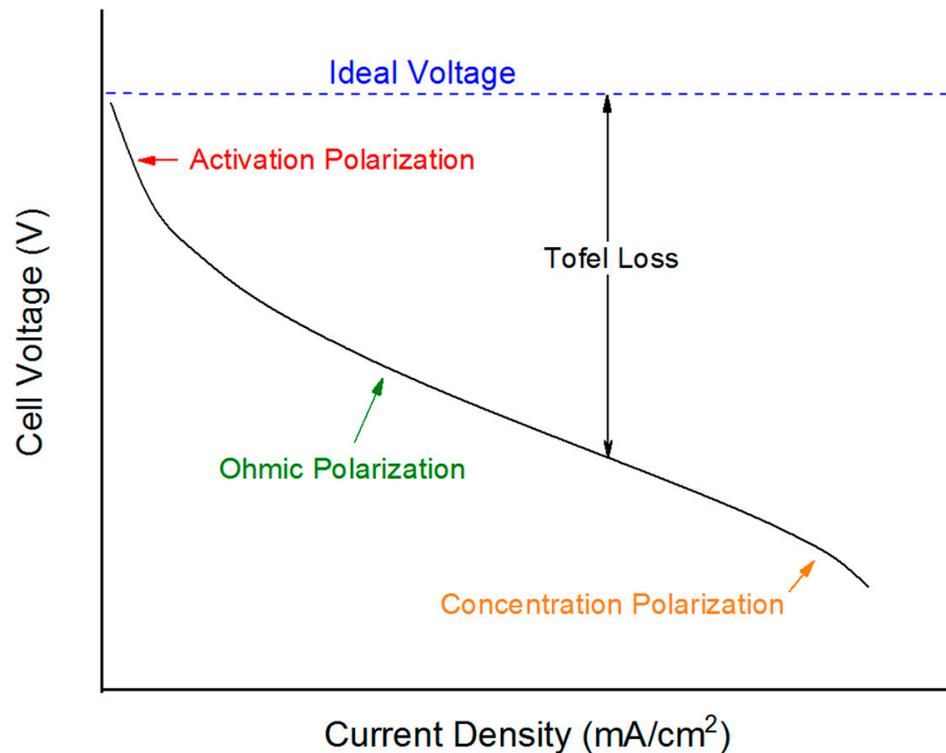
Figure 1. Fuel cell polarization curve.
