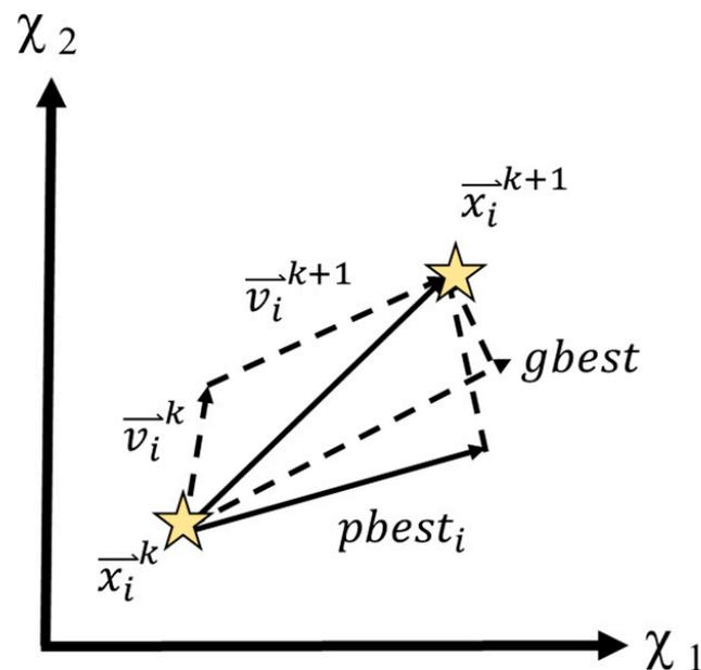
Figure 3. Particles changing positions through adjustment of their speed.
