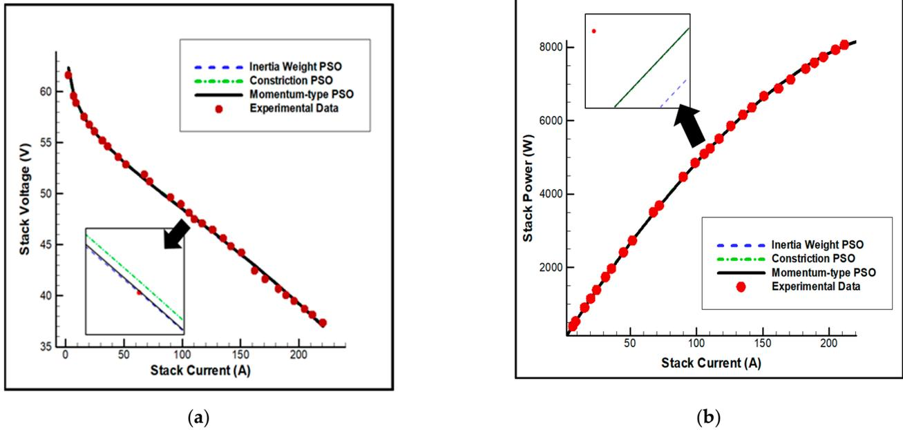
Figure 4. Calculation results of the PEMFC model: (a) I–V characteristic; (b) Power–V characteristic.
