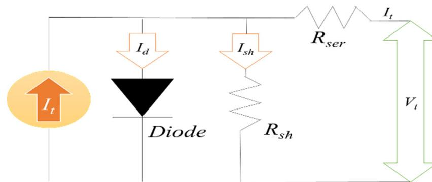
Figure 2. SD PV cell model.
