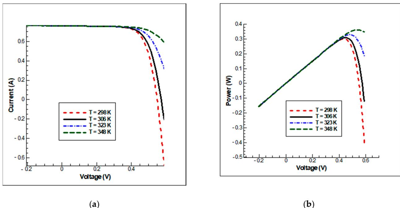
**Figure 8.** Effect of cell temperature on: (a) I–V characteristics; (b) Power–V characteristics in the SD model.
