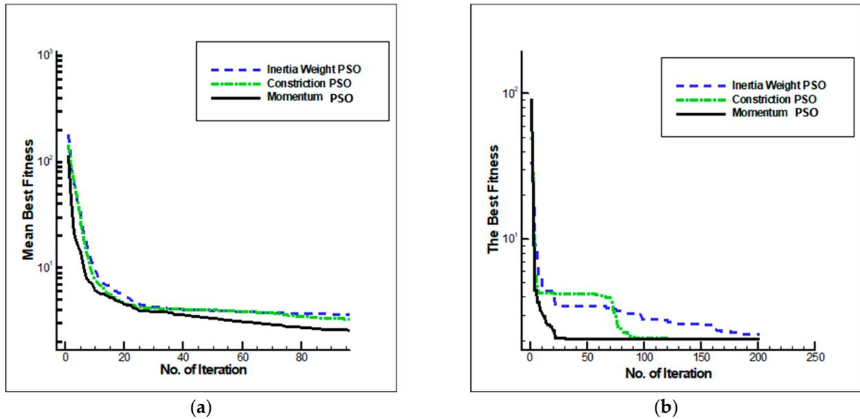
Figure 5. Convergent solutions: (a) Mean best solution convergence; (b) best solution convergence of the three improved PSO algorithms in the PEMFC model.
