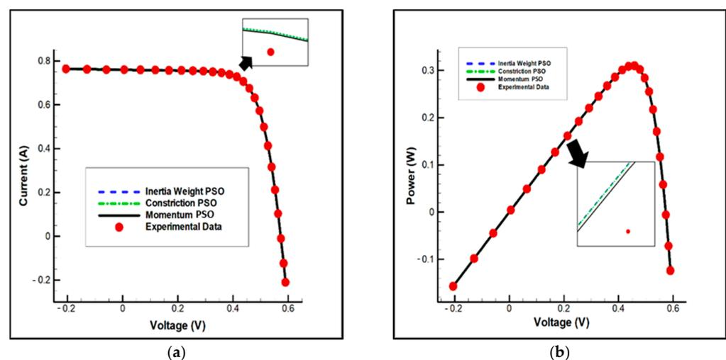
**Figure 6.** Curve analysis results of the three algorithms: (a) I–V characteristic; (b) Power–V characteristic calculation results of the SD model.
