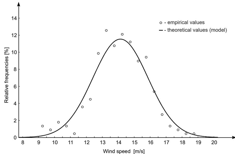
**Figure 6.** Empirical and theoretical probability density function of 110 kV overhead power lines resistance to load (exposure) in the form of wind occurring in their place of operation.
