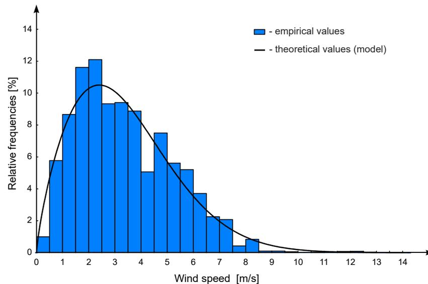
**Figure 5.** Empirical and theoretical wind speed probability density function at 110 kV overhead line locations.
