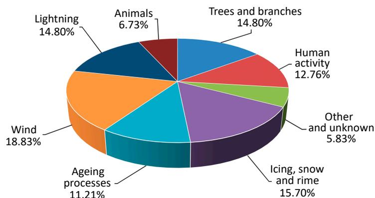
**Figure 1.** Percentage share of causes of 110 kV overhead line failures [4].
