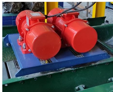
Figure 5. View of the support plate with MVE 510/1 vibrating motors mounted on the riddle of a WP screen.
