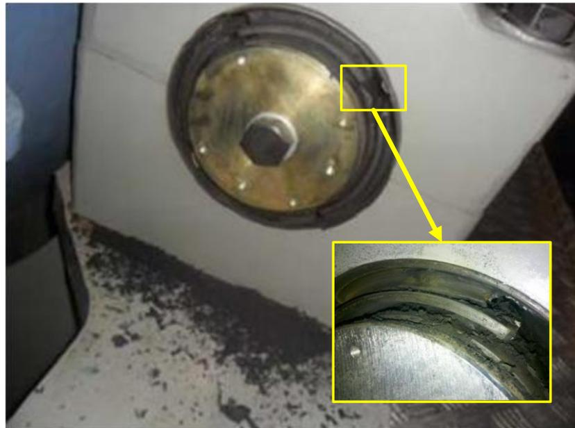
Figure 10. Main bearing offset failure.
