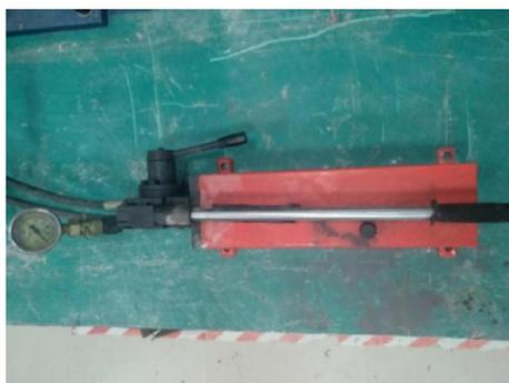
**Figure 7.** Manual hydraulic oil pump.
