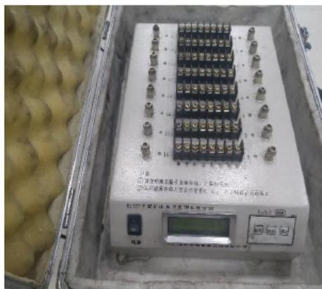
**Figure 9.** KJ327-F strain data collector.
