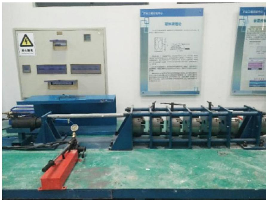
**Figure 5.** Physical diagram of the experimental device for the prestressed loading of the bolt.
