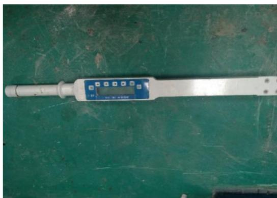
**Figure 6.** CML300 torque wrench.
