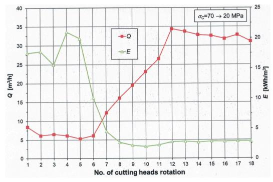
**Figure 12.** Mining efficiency (*Q*) and energy consumption (*E*) in subsequent rotations of the cutting heads during the performance of lower cut in the automatic control mode in rocks with decreasing uniaxial compressive strength.
