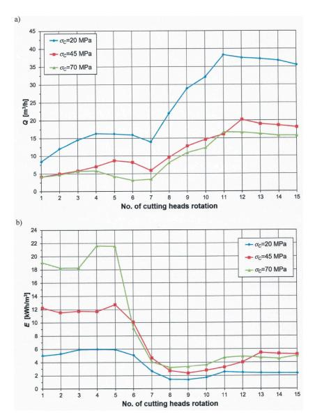
**Figure 6.** The course of: (a) mining efficiency (*Q*) and (b) mining energy consumption (*E*) in subsequent rotations of the cutting heads when making lower cuts in the automatic control mode in rocks with different uniaxial compressive strengths.
