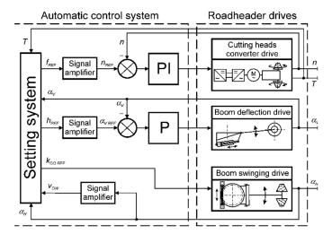
**Figure 2.** A simplified diagram of the automatic control system developed for controlling the cutting heads movement of a boom-type roadheader according to the proposed concept: n—rotational speed of the motor rotor driving the cutting heads,  $v_{OW}$ —movement speed of the cutting heads,  $\alpha_H \& \alpha_V$ —boom deflection angles in a plane parallel and perpendicular to the floor.
