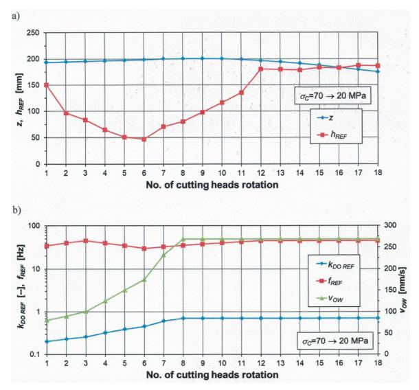
**Figure 10.** The course of cutting parameters: (a) web of cut (z) and set cut height ( $h_{REF}$ ) and (b) cutting heads movement speed ( $v_{OW}$ ), and set values: supply voltage frequency ( $f_{REF}$ ) and electrohydraulic valve opening coefficient ( $k_{DO\ REF}$ ) in subsequent rotations of the cutting heads when making lower cuts in the automatic control mode in rocks with decreasing uniaxial compressive strength.
