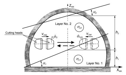
**Figure 9.** Scheme of mining a rock mass with a layered structure using parallel cuts to the floor of the drilled roadway.
