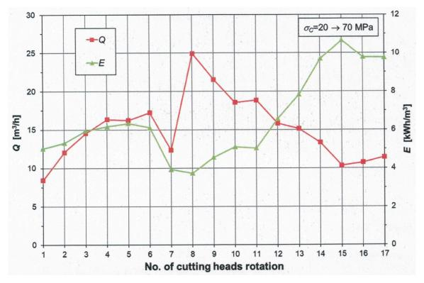
**Figure 15.** Mining efficiency (*Q*) and energy consumption (*E*) in subsequent rotations of the cutting heads during the performance of lower cut in the automatic control mode in rocks with increasing uniaxial compressive strength.
