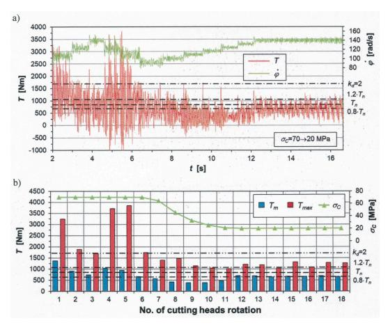
**Figure 11.** (a) Time courses of dynamic load on the motor shaft in the cutting heads drive (T) and its angular velocity  $(\dot{\varphi})$  and (b) values of parameters characterizing this load in subsequent rotations of the cutting heads during the performance of lower cut in the automatic control mode in rocks with decreasing uniaxial compressive strength.
