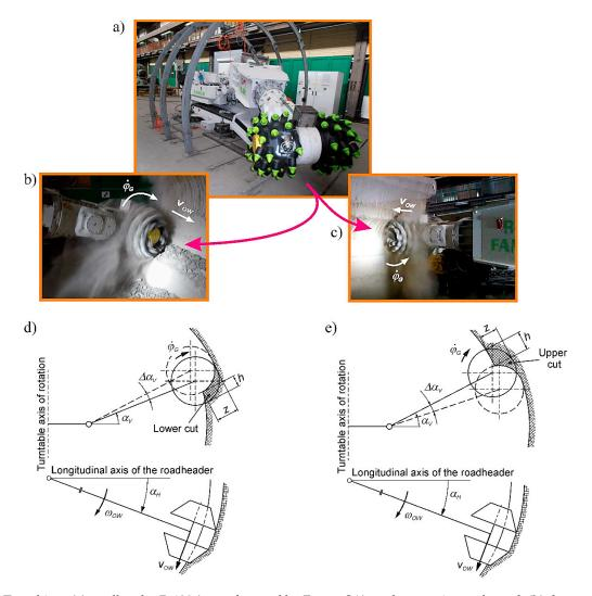
**Figure 1.** Test object: (a) roadheader R-130 (manufactured by Famur SA) on the experimental stand, (b) the course of the lower cut, (c) the course of the upper cut, (d) parameters characterizing the lower cut, and (e) parameters characterizing the upper cut.
