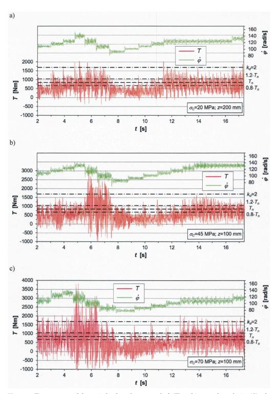
**Figure 5.** Time courses of dynamic load on the motor shaft (T) and its angular velocity ( $\dot{\varphi}$ ) when making lower cuts in the automatic control mode in rocks with uniaxial compressive strength ( $\sigma_C$ ) of: (a) 20 MPa, (b) 45 MPa, and (c) 70 MPa (the figures show the web of cut values for which cutting was simulated).
