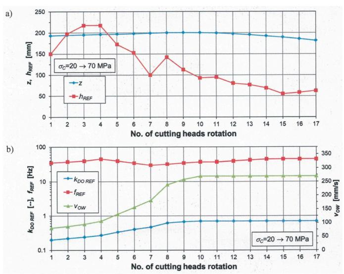
**Figure 13.** The course of cutting parameters: (a) web of cut (z) and set cut height ( $h_{REF}$ ) and (b) cutting heads movement speed ( $v_{OW}$ ), and set values: supply voltage frequency ( $f_{REF}$ ) and electrohydraulic valve opening coefficient ( $k_{DO\ REF}$ ) in subsequent rotations of the cutting heads during the performance of lower cut in the automatic control mode in rocks with increasing uniaxial compressive strength.
