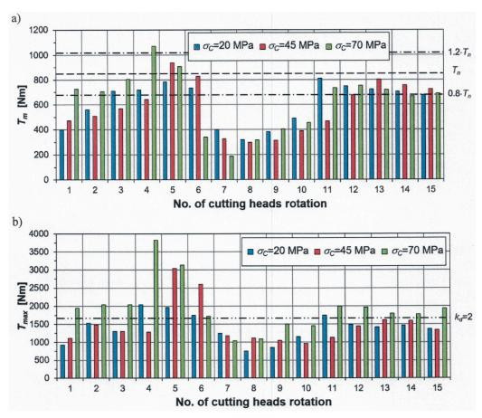
**Figure 4.** The course of: (a) the average value  $(T_m)$  and (b) the peak value  $(T_{max})$  of torque on the motor shaft in the cutting heads drive in subsequent rotations of the cutting heads when making lower cuts in the automatic control mode in rocks with different uniaxial compressive strengths.
