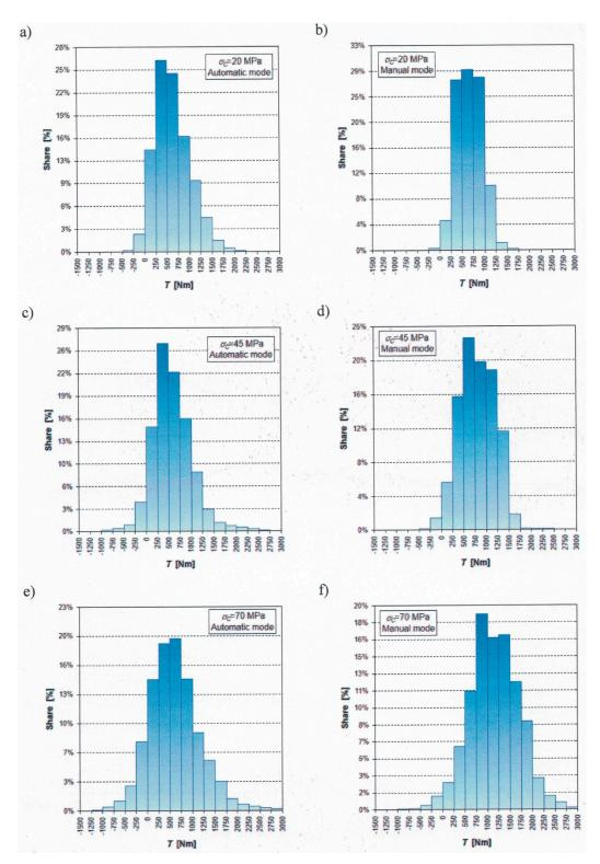
Figure 8. Histograms of the torque value distribution on the motor shaft in the cutting heads drive during simulated rock mining with three different uniaxial compressive strengths in (a,c,e) automatic control mode and (b,d,f) manual control mode.
