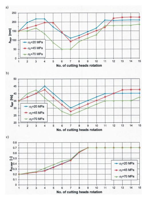
**Figure 3.** Setpoint values worked out by the setting system: (a) cut height  $(h_{REF})$ , (b) supply voltage frequency  $(f_{REF})$ , and (c) opening coefficient of the electrohydraulic valve  $(k_{DO\ REF})$  in subsequent rotations of the cutting heads when making lower cuts in automatic mode in rocks with different uniaxial compressive strengths.
