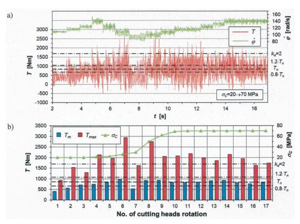
**Figure 14.** (a) Time courses of dynamic load on the motor shaft in the cutting heads drive (T) and its angular velocity  $(\dot{\varphi})$  and (b) values of parameters characterizing this load in subsequent rotations of the cutting heads during the performance of lower cut in the automatic control mode in rocks with increasing uniaxial compressive strength.
