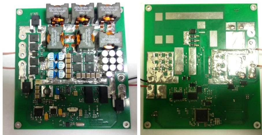
Figure 14. Step-down voltage converter of the power unit.
