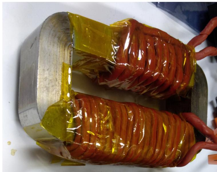
Figure 15. Transformer used in DAB converter.
