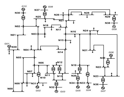
Figure 9. One-line diagram of the IEEE 39-bus system.
