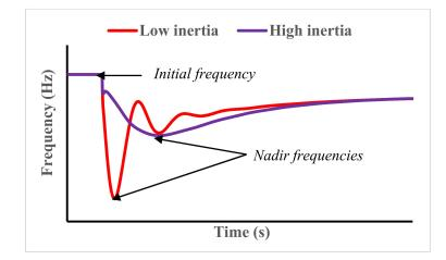
Figure 2. Frequency response under varying inertia.
