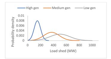
Figure 23. Load shedding density considering RES-DG output.
