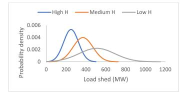
Figure 22. Load shedding density considering system inertia.
