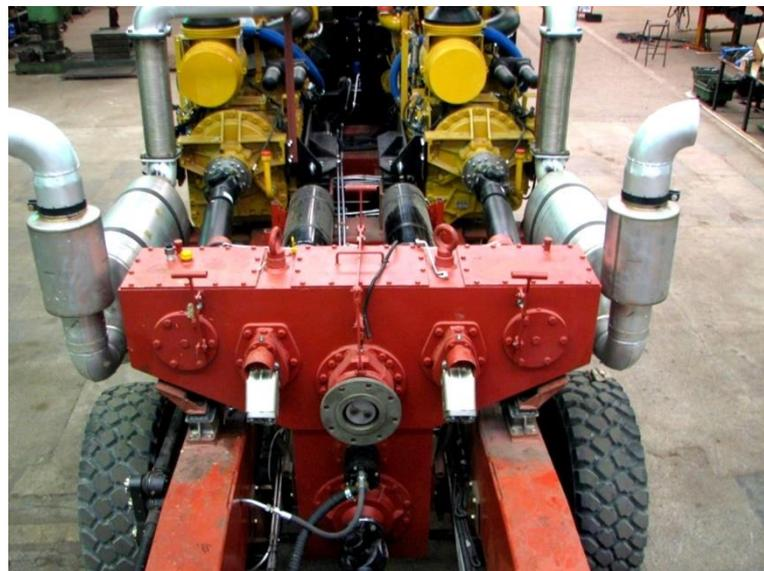
**Figure 2.** The adder and distribution box.
