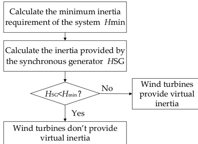
**Figure 2.** Decision of whether the wind turbines participate in the inertia response.
