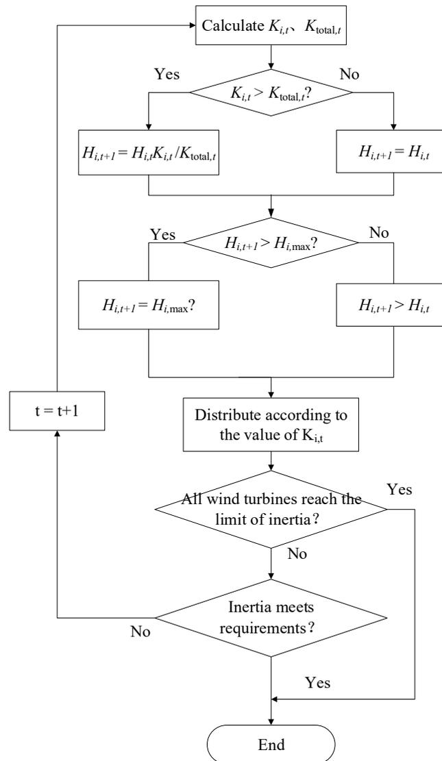
**Figure 4.** Flow chart of wind turbine inertia adjustment.
