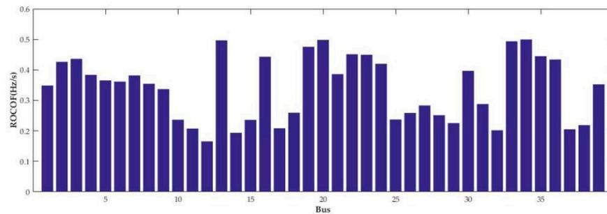
**Figure 7.** Rate of change in frequency of each node.
