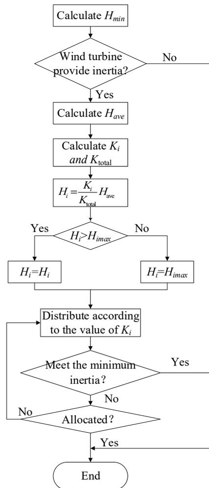
Figure 3. Flow chart of preliminary wind turbine inertia allocation.
