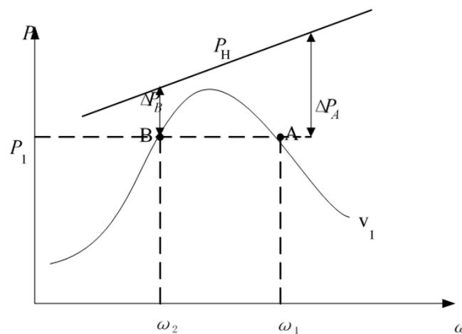
Figure 1. Power tracking curve of DFIG at different wind speeds.
