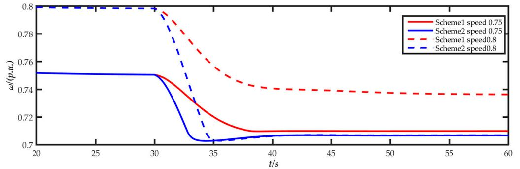
Figure 9. Speed change in wind turbines in the low-wind speed zone.
