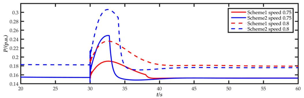
Figure 10. Power change in wind turbines in the low-wind speed zone.
