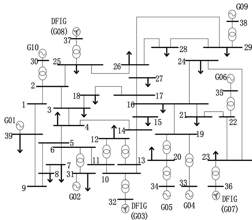
Figure 5. The modified IEEE 39-bus New England system.
