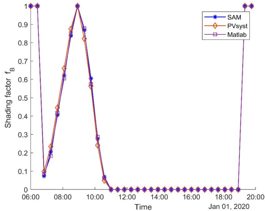
**Figure 15.** Shading factor  $f_B$  for situation 1 calculated for one day (1 January).  $f_B$  was calculated with the System Advisor Model (SAM), PVsyst, and the proposed Matlab tool.
