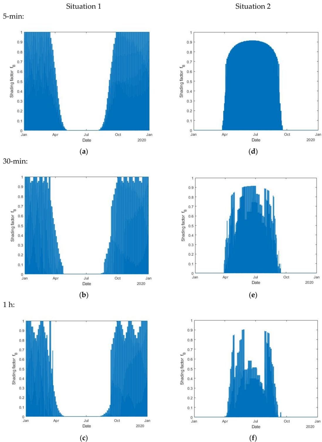
**Figure 17.** Effect of using different time steps when calculating the shading factor  $f_B$  with Matlab. For situation 1: (a) 5 min; (b) 30 min and (c) 1 h. For situation 2: (d) 5 min; (e) 30 min and (f) 1 h. As the time step increases, the yearly curve of  $f_B$  deteriorates and loses symmetry.
