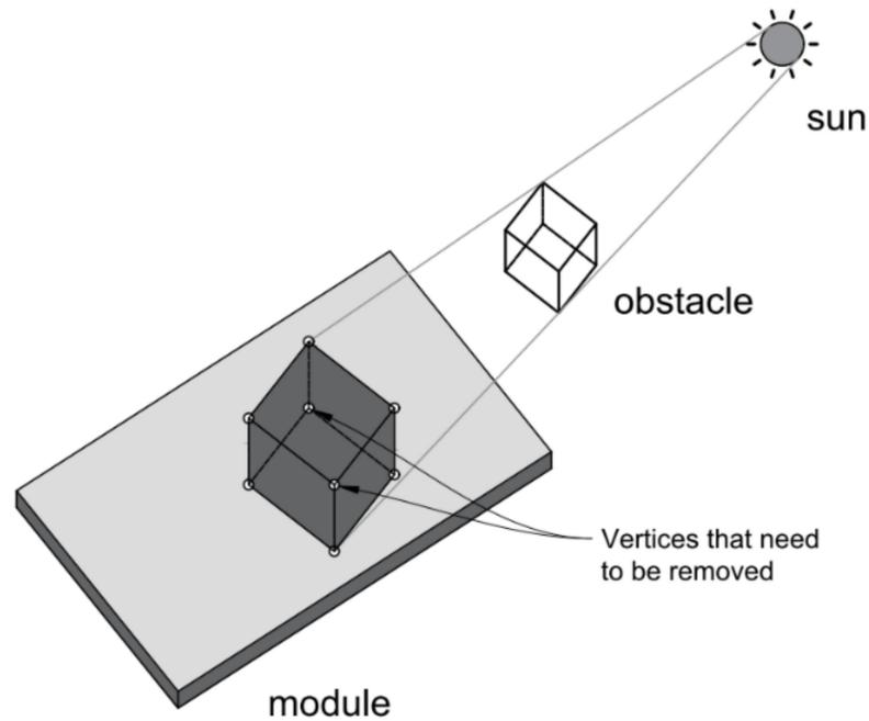
**Figure 6.** Projection of each of the eight obstacle vertices onto the surface of the module. After projecting all the points, there are two points that need to be removed. These two points are internal to the shadow and do not correspond to the ones located on the perimeter of the shadow.
