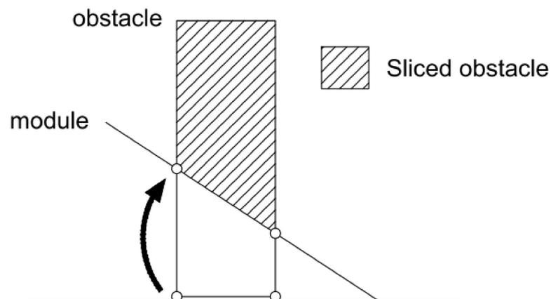
**Figure 5.** Side view of one module and one obstacle. If some of the obstacle vertices are behind the module plane, it is possible to slice the obstacle by moving these vertices vertically until they are positioned on the plane.
