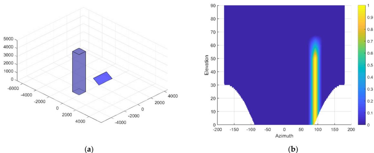
**Figure 13.** Situation 1, one PV module being shaded by one obstacle positioned on its east side with 2 m of separation. The tilt angle of the module is  $30^\circ$  and the azimuth angle is  $0^\circ$ : (a) Visual output; (b) Heat plot representation of the shading table.
