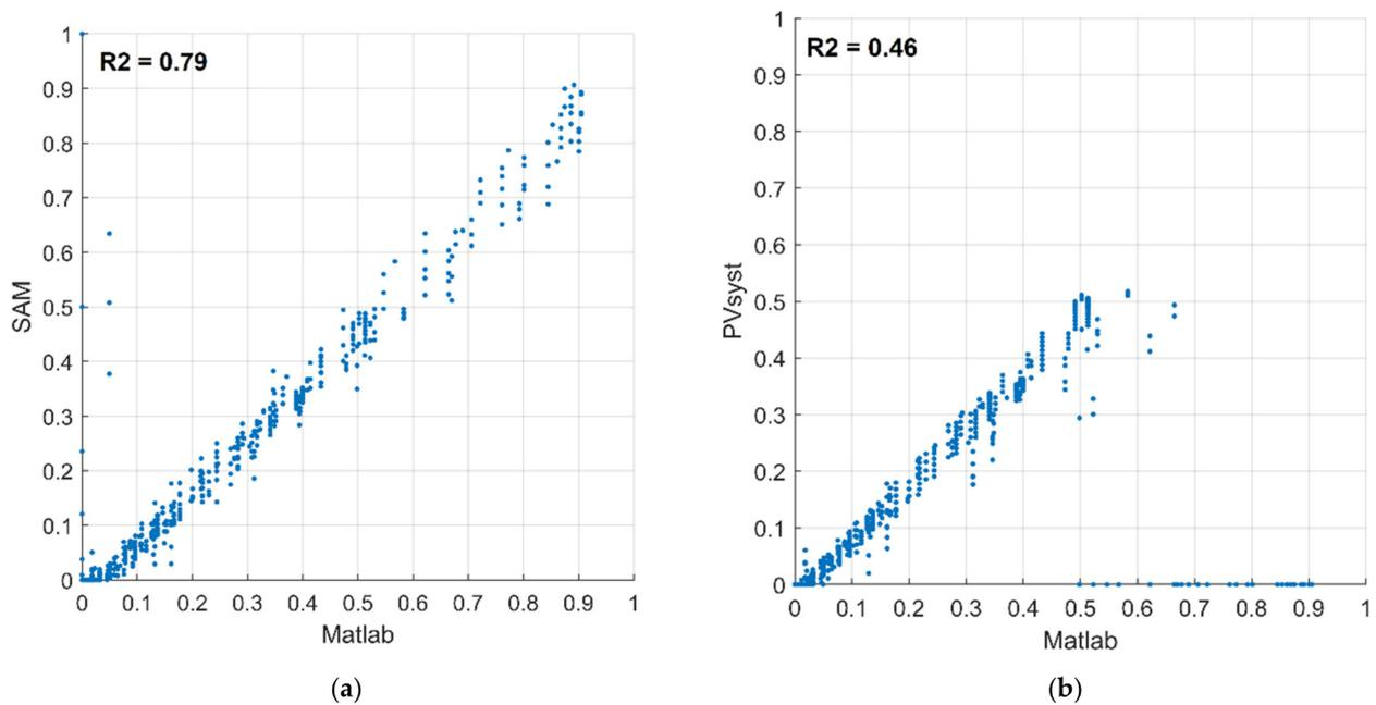
**Figure 20.** Scatter plots for the direct irradiance shading factor  $f_B$ . Comparison of: (a) Matlab with SAM and (b) Matlab with PVsyst. Results are for situation 2, one module shaded by one infinite row.
