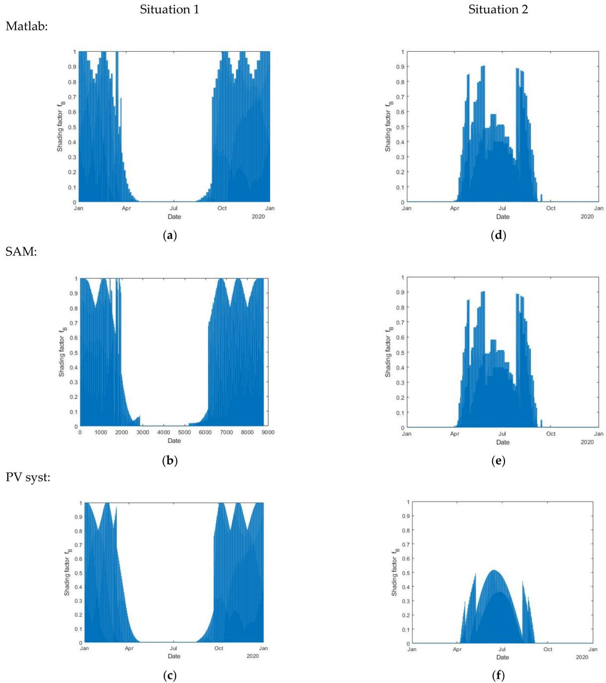
**Figure 18.** Shading factors  $f_B$  for a complete year. Results for situation 1 obtained with: (a) Matlab; (b) SAM and (c) PVsyst. Results for situation 2 obtained with (d) Matlab; (e) SAM and (f) PVsyst.
