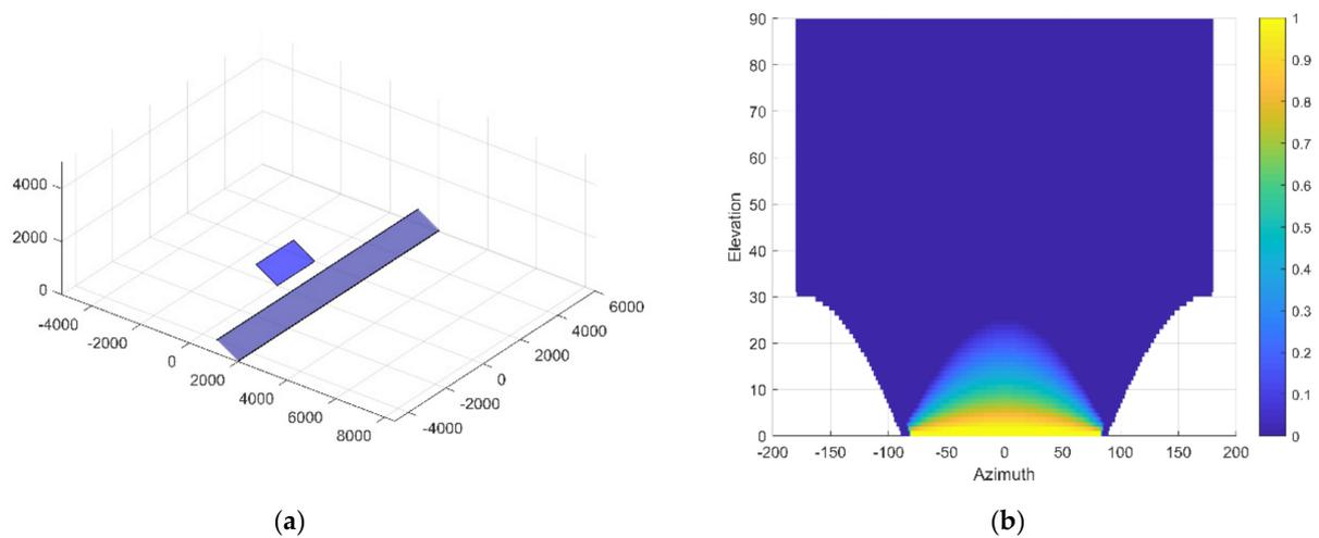
**Figure 14.** Situation 2, one PV module being shaded by one infinite row in front. The tilt angle of the row is  $30^\circ$  and is positioned at 2 m from the module. The tilt angle of the module is  $30^\circ$  and the azimuth angle is  $0^\circ$ : (a) Visual output; (b) Heat plot representation of the shading table.
