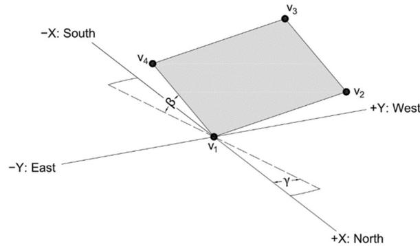
**Figure 2.** Geometric definition of the vertices  $v_1$ ,  $v_2$ ,  $v_3$ , and  $v_4$  for a solar module with tilt angle  $\beta$  and azimuth angle  $\gamma$ . Azimuth angles are measured from north and positive clockwise.
