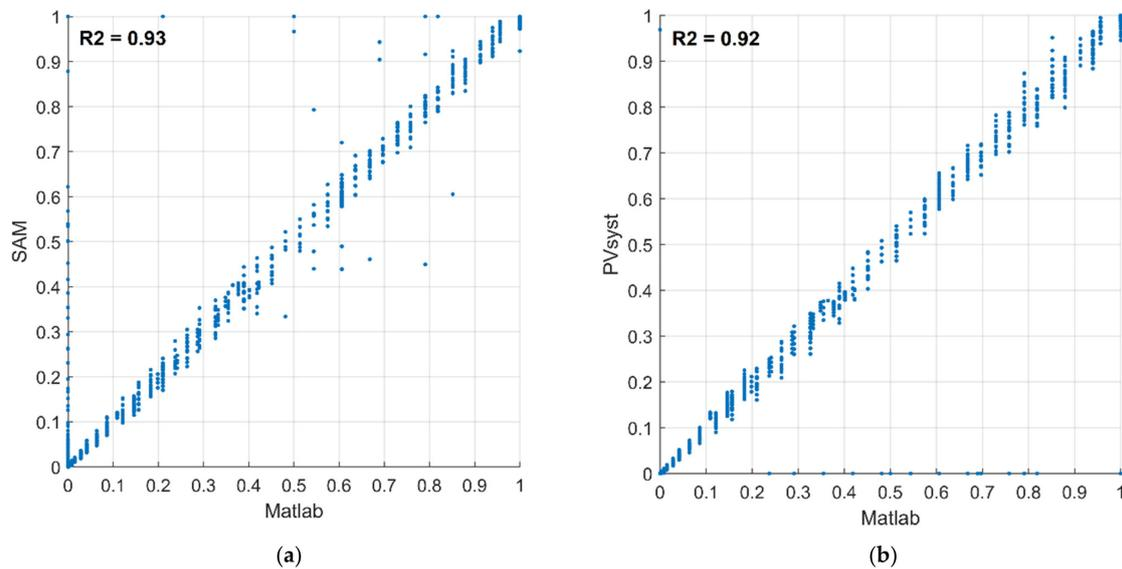
**Figure 19.** Scatter plots for the direct irradiance shading factor  $f_B$ . Comparison of: (a) Matlab with SAM and (b) Matlab with PVsyst. Results are for situation 1, one module shaded by a single obstacle positioned on the east side.
