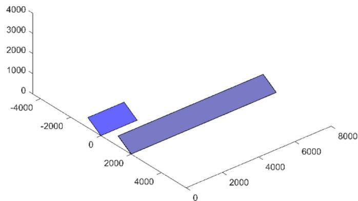
**Figure 12.** First module of the second row being shaded by the row in front. The shading factor for the inter-row shading is calculated for each module of the second row, being shaded by an obstacle with the size of the row in front.
