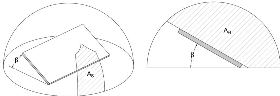
**Figure 10.** Calculation of the shading factor for the diffuse irradiance. If the solar module is covered by an imaginary hemisphere, then one nearby obstacle will reduce the diffuse irradiance reaching this hemisphere.  $A_S$  is the portion of the hemisphere where the sun is blocked by the obstacle. The diffuse irradiance shading factor is given as the ratio between the irradiance traversing  $A_S$  and the irradiance traversing the hemisphere  $A_H$ .
