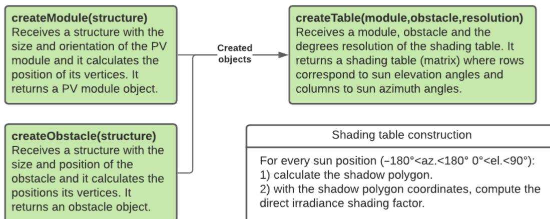
**Figure 1.** The classes createModule and createObstacle are used for creating the PV module and obstacle objects. The objects contain the geometry of the given situation. The class createTable receives the module, obstacle, and the angle resolution of the sun elevation and azimuth angles. Finally, the class returns a shading table object.
