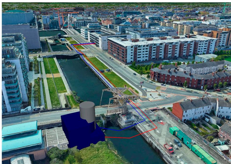
**Figure 6.** Depiction of a district energy plant located on the canal that uses a closed loop system to meet the summertime cooling needs of offices.
