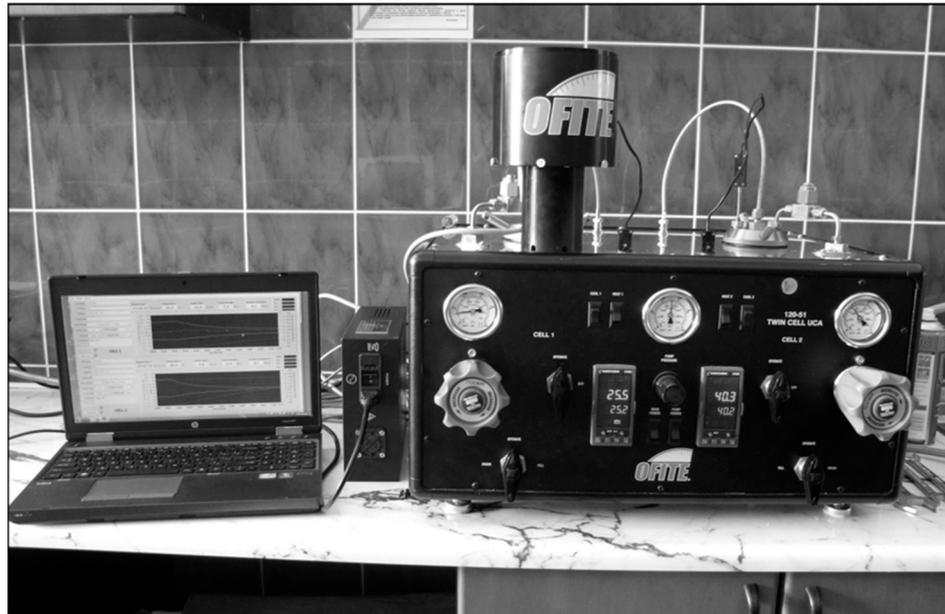
**Figure 6.** Apparatus for testing the build-up of static structural strength in slurry—two-chamber UCA SGSM Ofite model 120-53.
