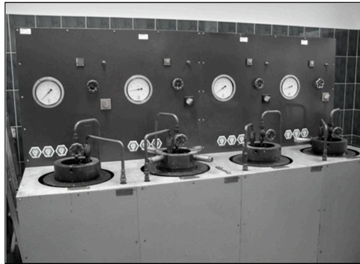
Figure 12. Autoclaves for storing samples of cement slurries.
