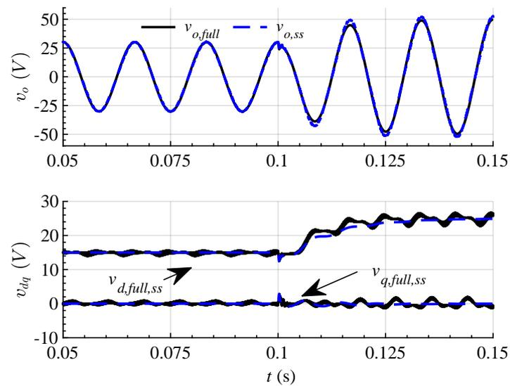
**Figure 18.** Comparison of the output voltages and the  $dq$  axis voltages from both the full order model and the small-signal model of the boost inverter. The  $d$  axis reference jumps from 15 V to 25 V and the  $q$  axis reference remains fixed at 0 V.
