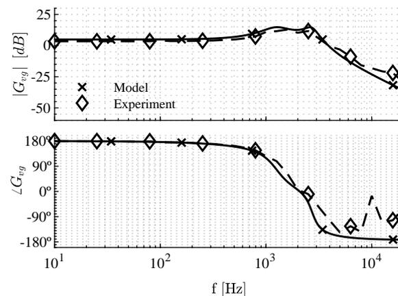
**Figure 9.** Bode plot comparison of audio susceptibility at  $D = 0.7$ . The results obtained from the small-signal line-to-output transfer function is compared with that of the one obtained from the experimental test bed.
