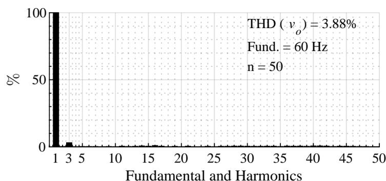
Figure 30. Measurement of harmonics and THD.
