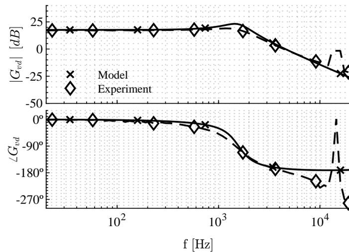
**Figure 11.** Bode plot comparison of control-to-output transfer function from the small-signal model and experimental test bed.
