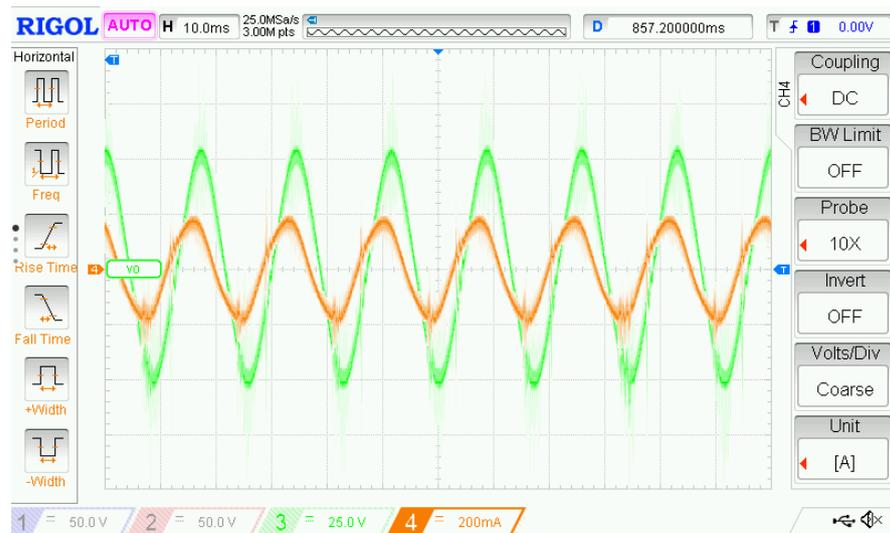
Figure 26. Measurement of output voltage and output current with an RC load.
