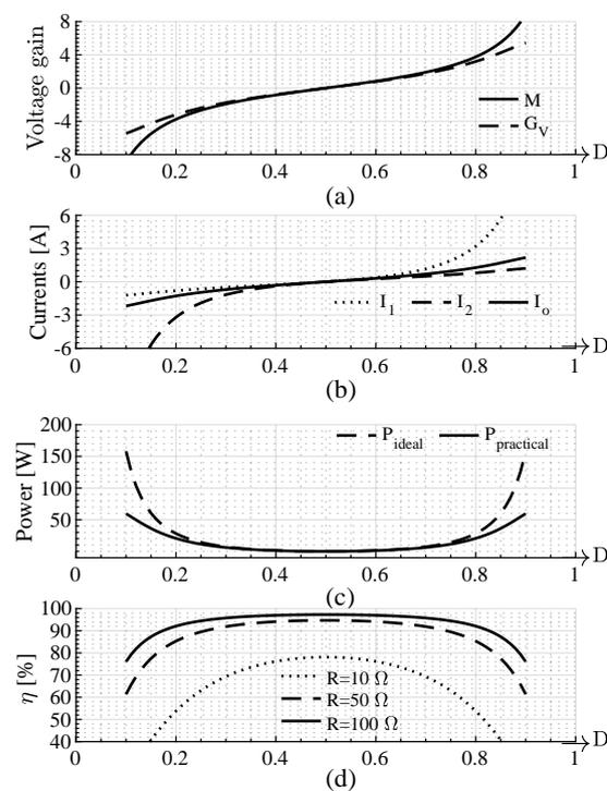
**Figure 6.** The characteristic plots obtained from the steady-state equivalent model as the duty cycle is varied: (a) Voltage gain with and without parasitic losses included, (b) individual converter and inverter currents, (c) inverter power considering the conduction losses only, and (d) efficiency considering the conduction losses only for three different load values as the duty cycle is varied.
