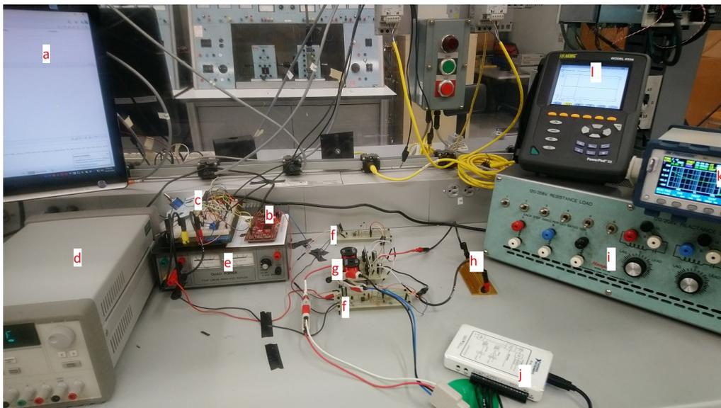
**Figure 22.** Experiment testbed. (a) Code composer studio, (b) TI DSP, (c) sensor board, (d) DC power supply for the inverter, (e) sensor board power supply, (f) gate driver boards, (g) inverter, (h)  $50\ \Omega$  load, (i) RLC load, (j) NI myDAQ for verification of  $G_{vg}$  and  $G_{vd}$ , (k) BK precision LCR meter for impedance verification, and (l) AEMC power quality analyzer.
