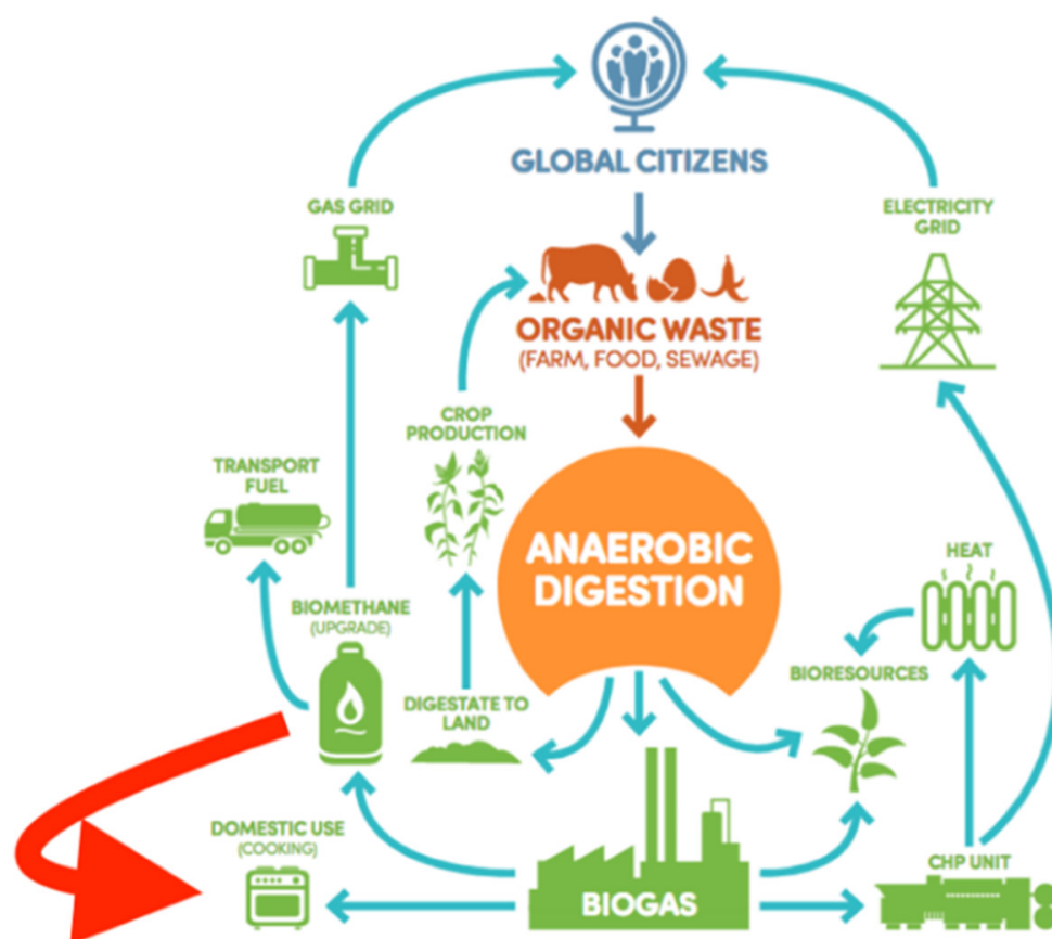
Figure 1. Anaerobic digestion systems and the proposed opportunity for compressed and bottled biogas (modified from [3]).
