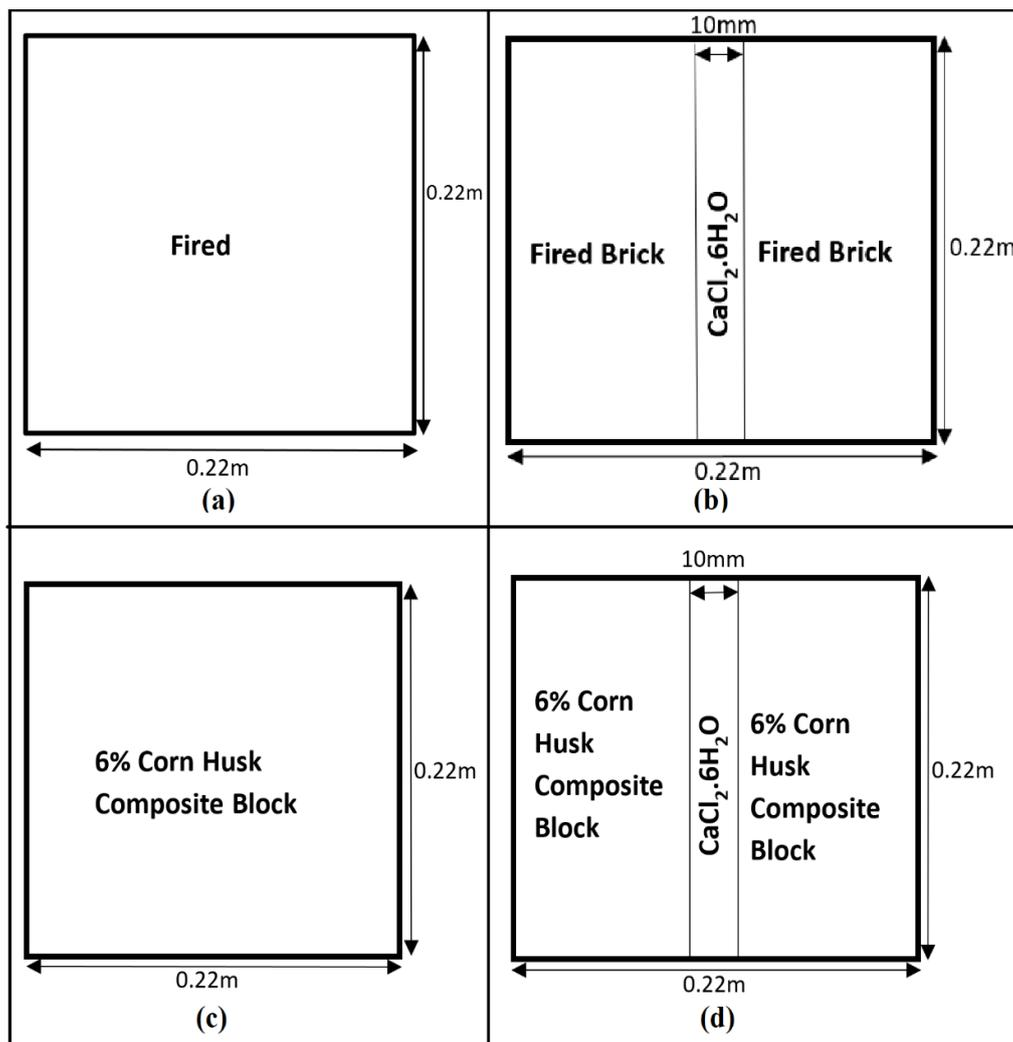
**Figure 16.** Model of fired brick and 6% corn husk composite block walls (a–d) with and without PCM.
