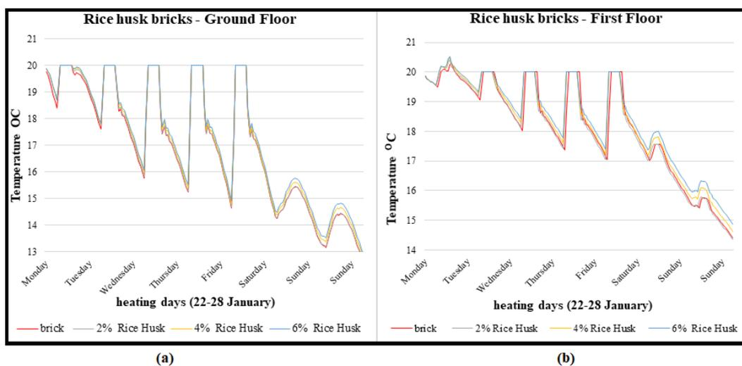
**Figure 11.** Ground (a) and first floor (b) heating loads using rice husk composite bricks.
