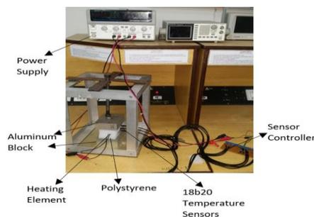
**Figure 5.** Experimental setup for thermal conductivity measurement [49,50]. This work is available online under the Creative Commons Attribution 3.0 IGO license (CC BY 3.0 IGO) <https://creativecommons.org/licenses/by/3.0/igo/>, accessed on 13 June 2021.
