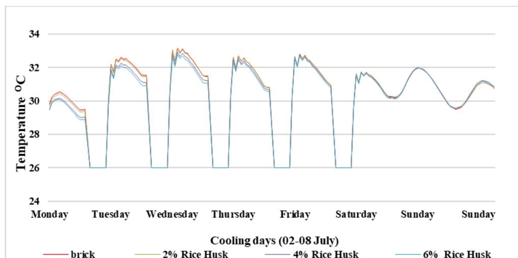
Figure 14. First-floor cooling load using rice husk composite bricks.
