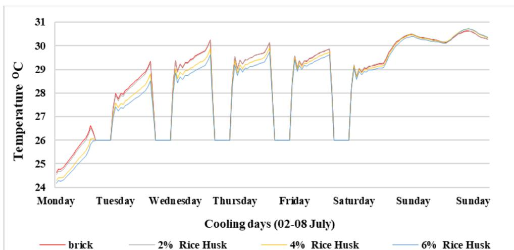
Figure 13. Ground floor cooling load using rice husk composite bricks.
