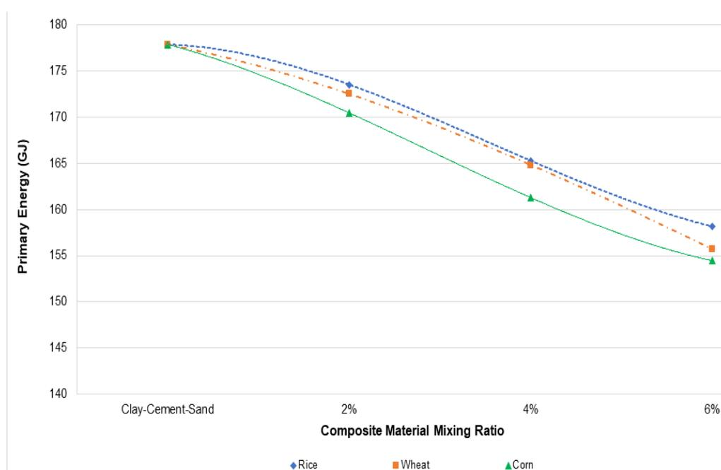
**Figure 12.** Heating load comparison using different composite materials and mixing ratios.
