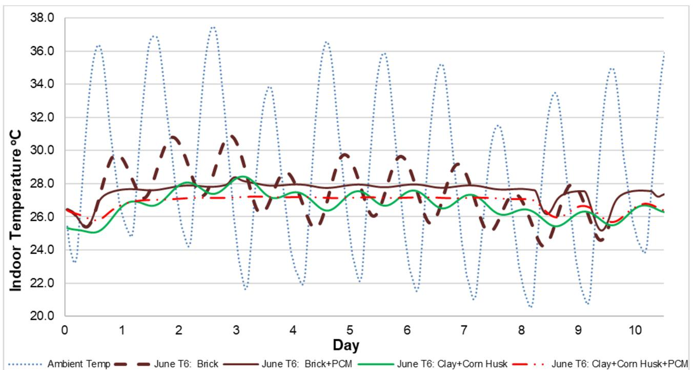
**Figure 17.** Simulation results depicting indoor temperature variation with outdoor ambient conditions.
