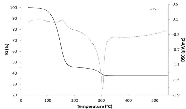
Figure 4. TG–DSC analysis of one of the inks produced.
