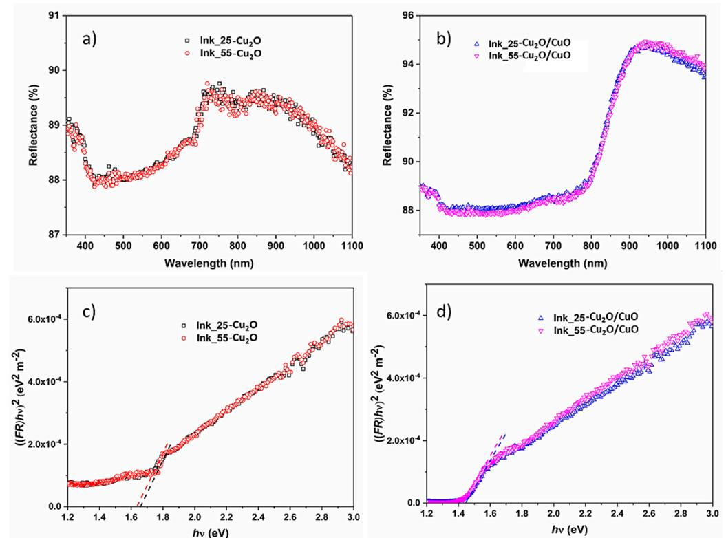
**Figure 8.** UV–Vis diffuse reflectance spectra of films produced with  $\text{Cu}_2\text{O}$ -based ink (a) and  $\text{Cu}_2\text{O}/\text{CuO}$ -based ink (b), and related Tauc plots for  $\text{Cu}_2\text{O}$ -based ink (c) and  $\text{Cu}_2\text{O}/\text{CuO}$ -based ink (d).
