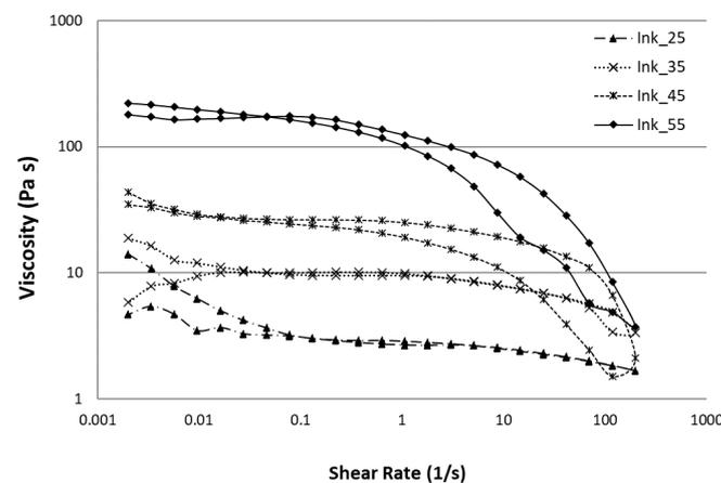
**Figure 3.** Flow curves of the formulated CuO inks.
