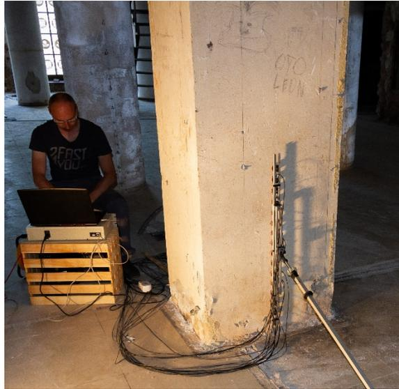
**Figure 3.** The building of the Heimann’s Foundation in Wrocław: internal pillar with EIT electrodes on opposite sides.
