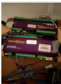
Figure 6. Data acquisition system (DT 500 datalogger).
