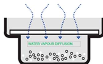
Figure 3. Diagram of dry cup test method [13].
