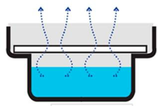
Figure 2. Diagram of wet cup test method [13].
