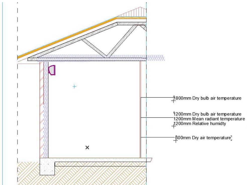
Figure 5. Architectural section of test building.
