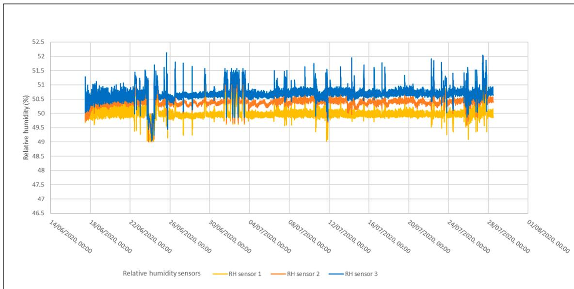
**Figure 22.** Relative humidity profile of the room aimed at 50% for the testing period 2.
