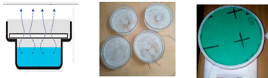
Figure 17. Wet-cup test method.
