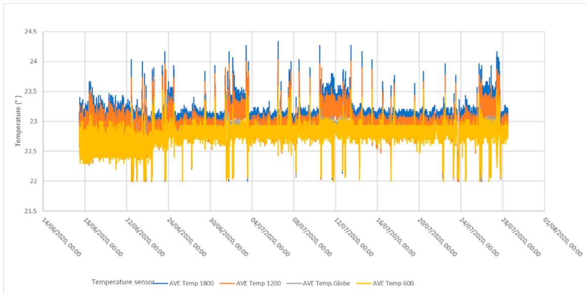
**Figure 21.** Temperature profile of the room aimed at 23 °C ( $\pm 0.5$  °C) for the testing period 2.
