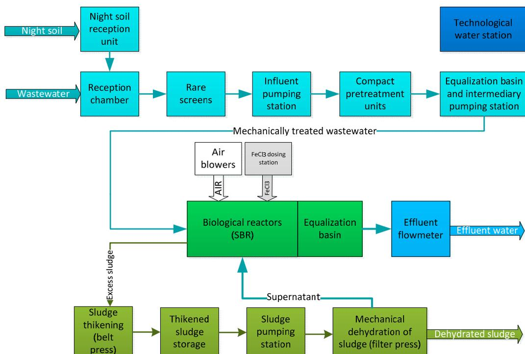
Figure 2. Process flow diagram for WWTP.
