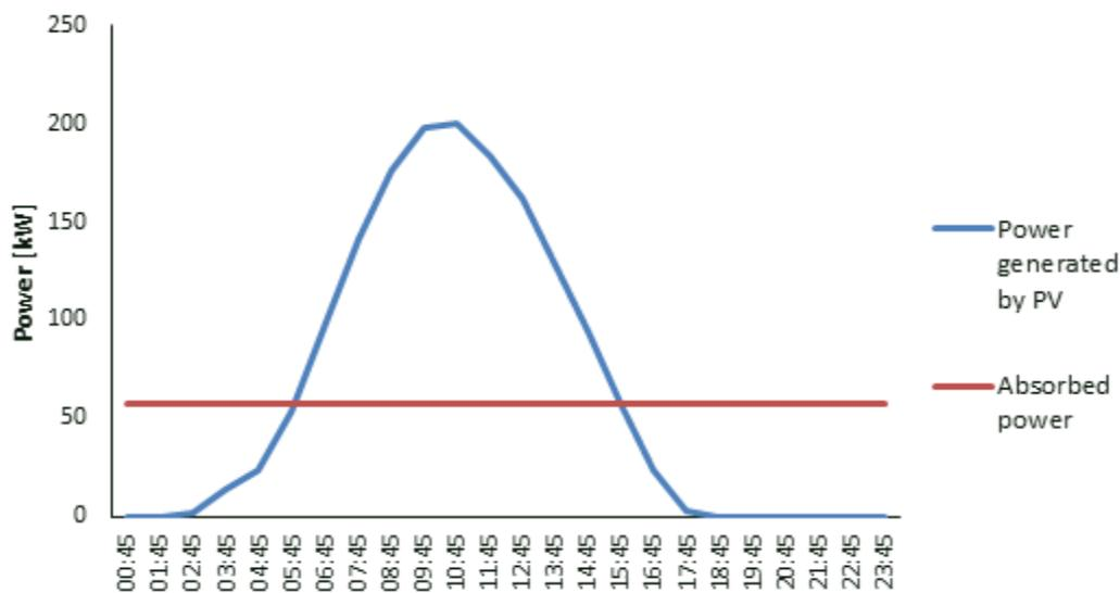
Figure 6. Hourly average power of WWTP for a typical day in July.
