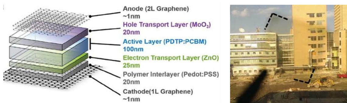
**Figure 3.** Axonometric view of the device structure; Photograph taken through a device, with dotted lines outlining device corners. Reproduced from [37], with permission from John Wiley & Sons Inc. (2016).
