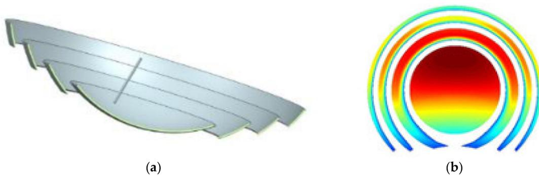
**Figure 5.** Definition of the solar field for a MOSAIC module: (a) Schematic cross-section showing a central bowl and three rings beside a cylindrical receiver; (b) Annual contribution for a given configuration and tilt angle. The southern mirrors contributing less have been removed.
