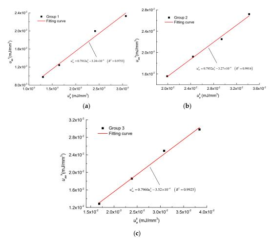
**Figure 7.** Relationship between elastic strain energy density and total input strain energy density for PJ coal mine: (a) Group 1; (b) Group 2; (c) Group 3.
