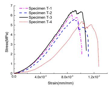
Figure 11. Stress-strain curves of four typical specimens in TJH coal mine.
