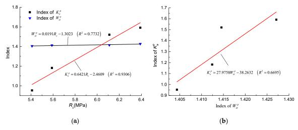
**Figure 15.** Relationship between different parameters in TJH coal mine: (a) Indexes  $K_e^p$ ,  $W_{et}^p$ , and UCS; (b) indexes  $K_e^p$  and  $W_{et}^p$ .
