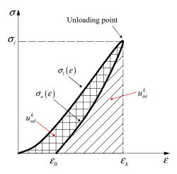
Figure 1. Calculation of elastic strain energy index.
