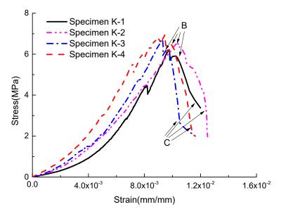
Figure 8. Stress-strain curves of coal specimens under uniaxial compression condition.
