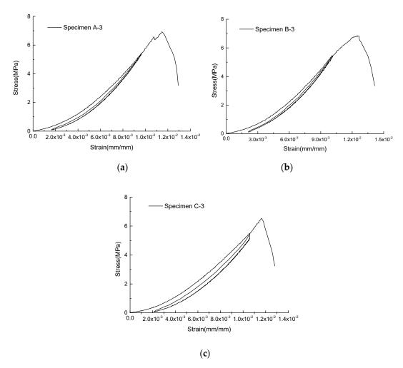
**Figure 6.** Representative loading-unloading stress–strain curves for each group: **(a)** Specimen A-3; **(b)** Specimen B-3; **(c)** Specimen C-3.
