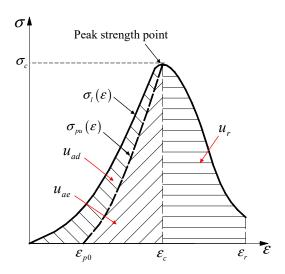
Figure 3. Calculation of modified bursting energy index.
