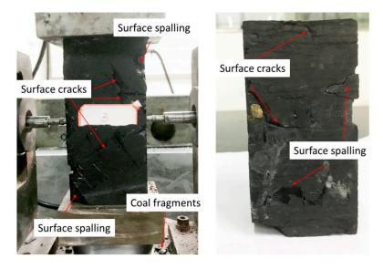
Figure 12. Ultimate failure mode of coal specimens in TJH coal mine.
