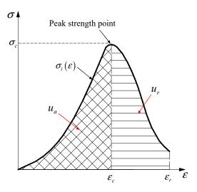
Figure 2. Calculation of bursting energy index.
