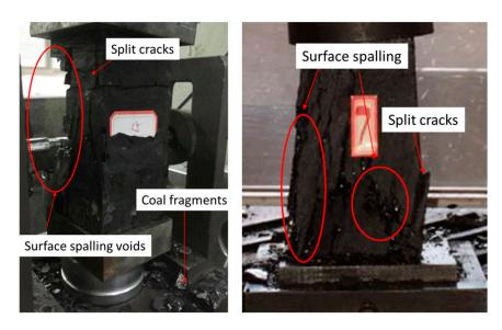
Figure 9. Ultimate failure mode of coal specimens in PJ coal mine.
