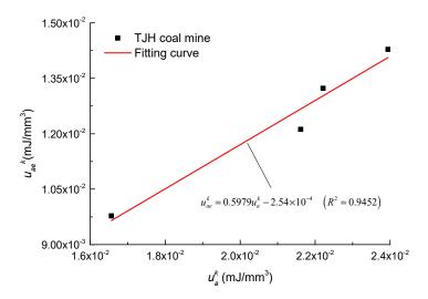
**Figure 10.** Relationship between elastic strain energy density and total input strain energy density for TJH coal mine.
