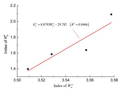
**Figure 14.** Relationship between indexes  $K_e^p$  and  $W_{et}^p$  in PJ coal mine.
