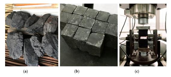
**Figure 5.** Coal specimens laboratory test procedures: (a) Coal blocks; (b) standard coal specimens; (c) Loading tests on RMT-150C.
