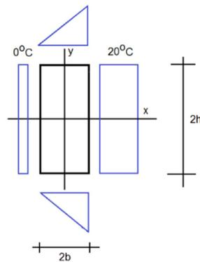
Figure 7. Steady-state temperature on the edges of Plate 2.
