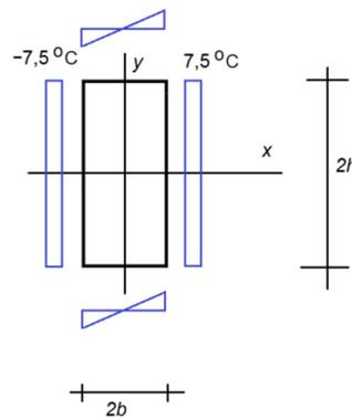
Figure 5. Antisymmetric part relative to  $x$  and symmetric to  $y$ . AS state.
