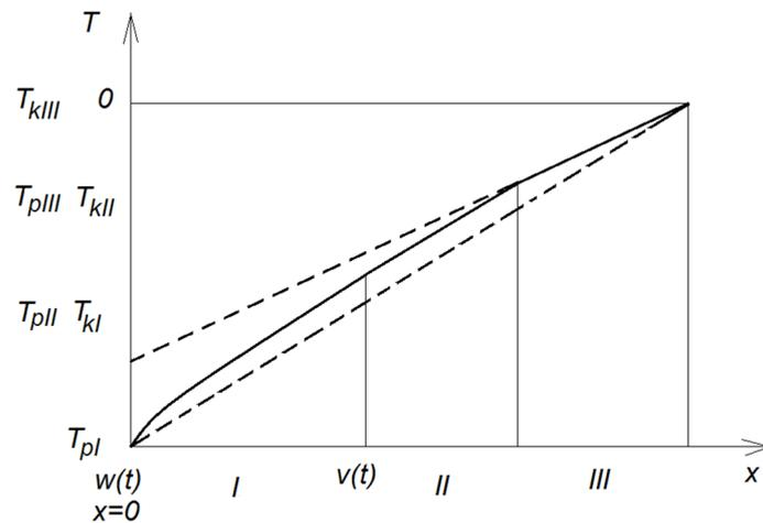
**Figure 11.** Temperature function on the sections  $w(t) \leq x < v(t)$  and  $v(t) \leq x < g$  caused by an impulse.
