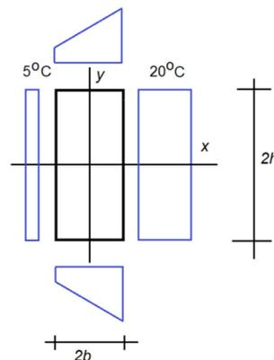
Figure 3. Example of boundary conditions of temperature in the shield.
