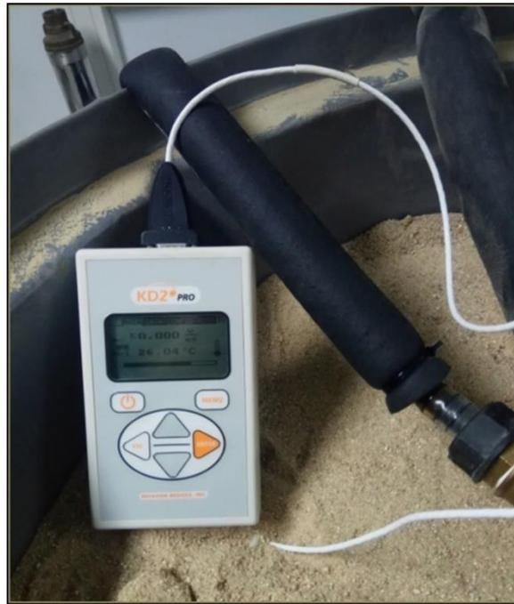
**Figure 12.** Measuring the ground thermal conductivity using KD2 Pro equipment and RK-1 sensor.
