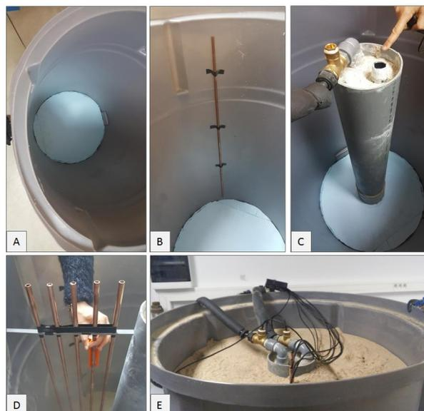
Figure 2. Installation of the experimental setup: (A) Thermal insulation of the main container, (B) main container and first copper tube, (C) geothermal borehole placement, (D) Set of copper tubes set to equal distances, and (E) overview of the setup with all the sensors and accessories.
