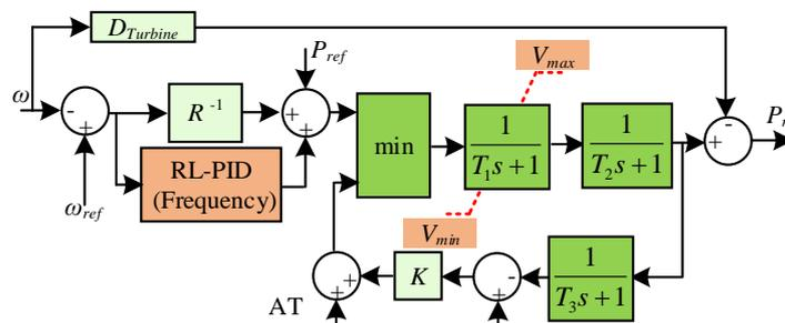
**Figure 13.** The modified model of the gas turbine of combined heat and power (CHP) with an extra adaptive controller [57].
