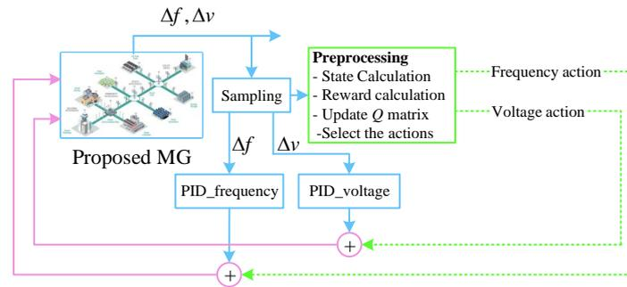
Figure 10. The implementation idea of the proposed control method based on RL.
