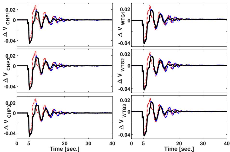
**Figure 17.** The oscillations of voltage at the generator buses in *scenario 1*; black(solid): RL-PID, blue (dashed–dotted): F-PID, red (dotted): PID.
