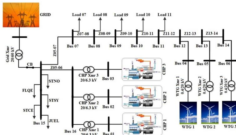
Figure 11. The single line diagram of the proposed real micro-grid (MG).
