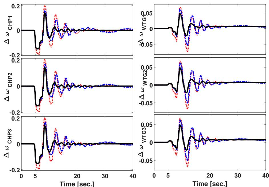
**Figure 16.** The oscillations of the angular velocity of generation units in *scenario 1*; black(solid): RL-PID, blue(dashed-dotted): F-PID, red(dotted): PID.
