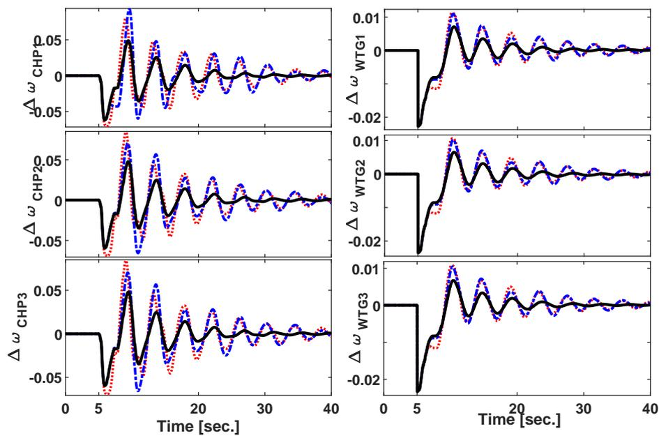
**Figure 18.** The oscillations of the angular velocity of generation units in *scenario 2*; black(solid): RL-PID, blue (dashed–dotted): F-PID, red (dotted): PID.
