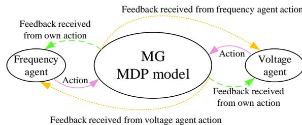
**Figure 5.** The proposed game-theory based reinforcement learning (RL) framework description considering the frequency and voltage agents.
