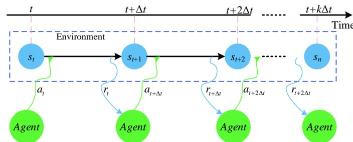
**Figure 9.** The operating process of the agent in a discrete environment in time steps.
