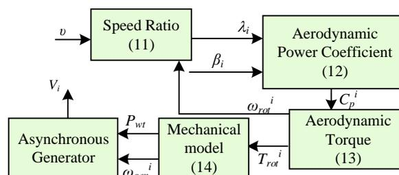
Figure 12. Conceptual model of the Fixed-speed wind generator [57].
