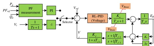
**Figure 14.** The modified IEEE’s type AC5A with secondary voltage controller.
