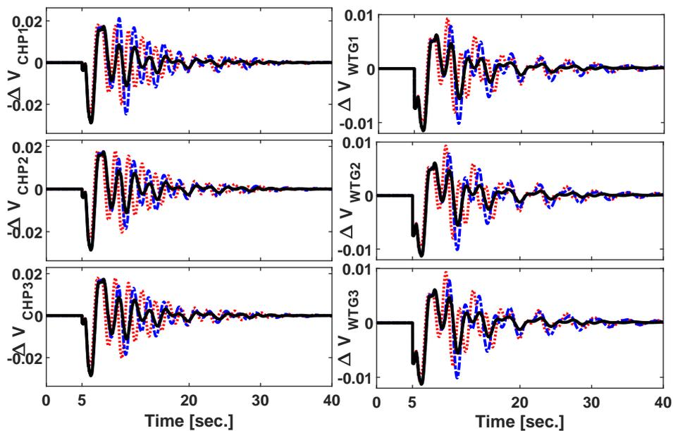
**Figure 19.** The oscillations of voltage at the generator buses in *scenario 2*; black(solid): RL-PID, blue (dashed–dotted): F-PID, red (dotted): PID.
