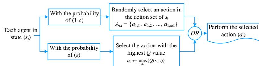
**Figure 3.** The  $\epsilon$ -greedy mechanism for selecting the proper action.
