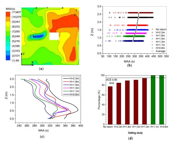
**Figure 10.** Mean air age (MAA) values distribution and a air change efficiency (ACE) percentage: (a) MAA value of H = 1.5 m setting at the Plane Z = 1.0; (b) Comparison of MAA values for seven settings at the Plane Z = 1.0; (c) MAA values profile along the room height in the vicinity of occupants; and, (d) ACE percentage in Plane Z = 1.0.
