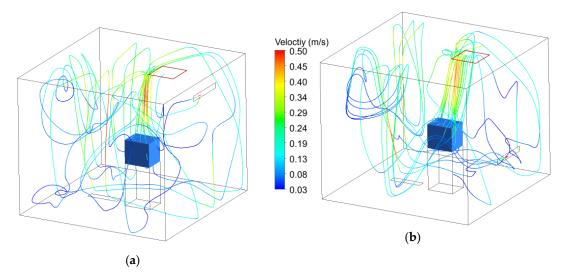
Figure 11. Air path line from the CO<sub>2</sub> source: (a) H = 2.3 m setting; and, (b) H = 0.8 m setting.
