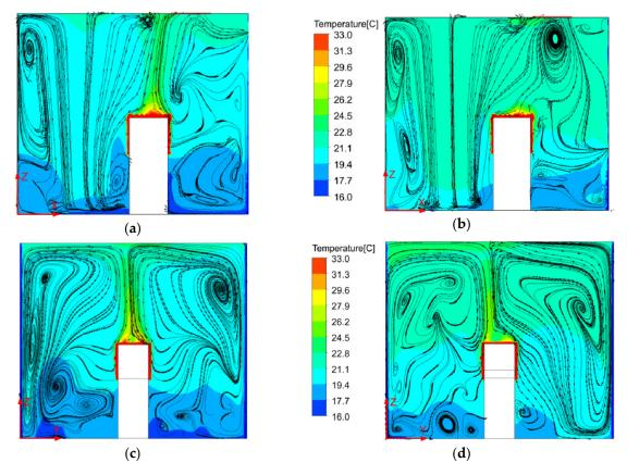
**Figure 4.** Temperature and streamline distributions for (**a**) H = 2.3 m setting at the Plane Y = 0; (**b**) H = 0.8 m setting at the Plane Y = 0; (**c**) H = 2.3 m setting at the Plane X = 1.8; and, (**d**) H = 0.8 m setting at the Plane X = 1.8.
