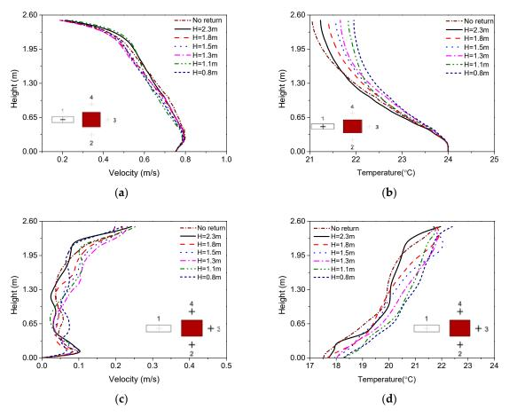
**Figure 5.** Effects of the return vent height on the air velocity and temperature profiles: (**a**,**b**) along Line 1 (**c**,**d**) in the vicinity of heaters.
