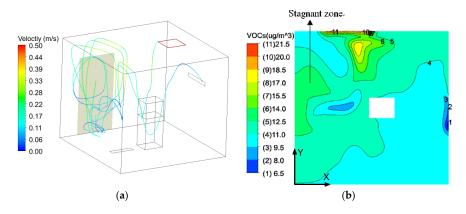
**Figure 13.** Air streamline and volatile organic compounds (VOCs) concentration of H = 1.5 m setting: (a) air path line started from VOCs source; (b) distribution of VOCs concentration at the Plane Z = 1.0.
