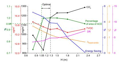
Figure 1. Comprehensive indices at different height of return air vent in cooling mode.
