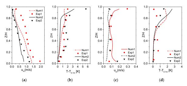
**Figure 3.** The comparison of simulated air velocity and temperature against the experimental data: (**a**,**b**) Jet centerline; (**c**,**d**) Free area ( $T_{0.1 \text{ m}}$  is air temperature at 0.1 m height)
