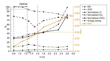
**Figure 15.** Comprehensive indices at different height of return air vent in heating mode. Note: *Normalized*  $\Delta T = \frac{\Delta t_{head-ankle}}{3}$ ; normalized concentration  $C_n = \frac{C_p}{C_e} C_p$  = concentration of contaminant in breathing zone;  $C_e$  = concentration of contaminant in exhaust [8,40].
