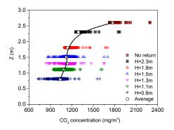
**Figure 12.** Comparison of frequency distribution of  $CO_2$  concentration for seven settings at breathing level (Plane Z = 1.0).
