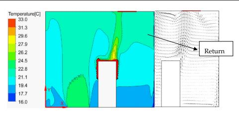
Figure 8. Temperature and Velocity distribution at the Plane Y = 0 (Case H = 1.5 m).
