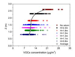
**Figure 14.** Comparison of frequency distribution of VOCs concentration for seven settings at breathing level (Plane Z = 1.0).
