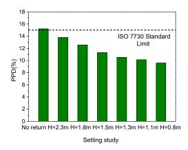
Figure 7. Predicted percentage dissatisfied (PPD) index for different settings.
