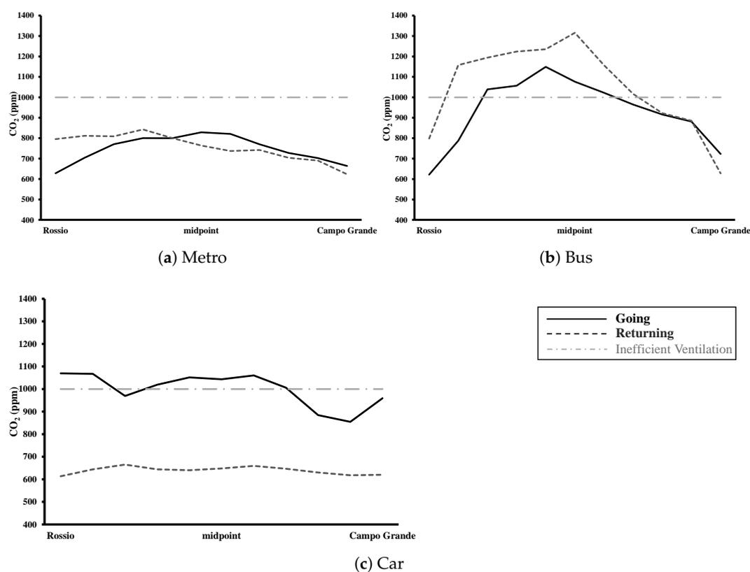
**Figure 5.** Temporal analysis of CO<sub>2</sub>. The dashed line is read from right to left. The dash-dotted line represents the threshold for efficient ventilation of 1000 ppm [33].
