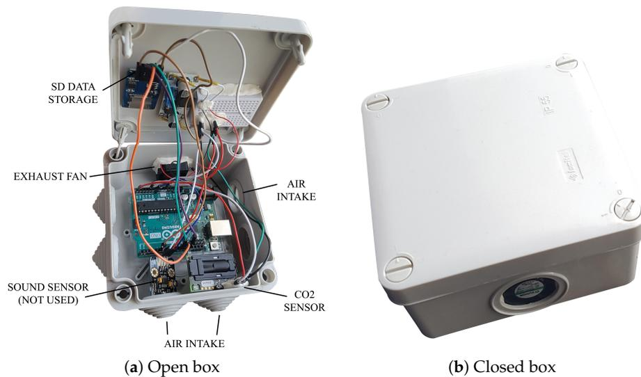
**Figure 2.** Box with  $105 \times 105 \times 55$  mm dimensions containing all the components in Table 1 except the smartphone and smartwatch.
