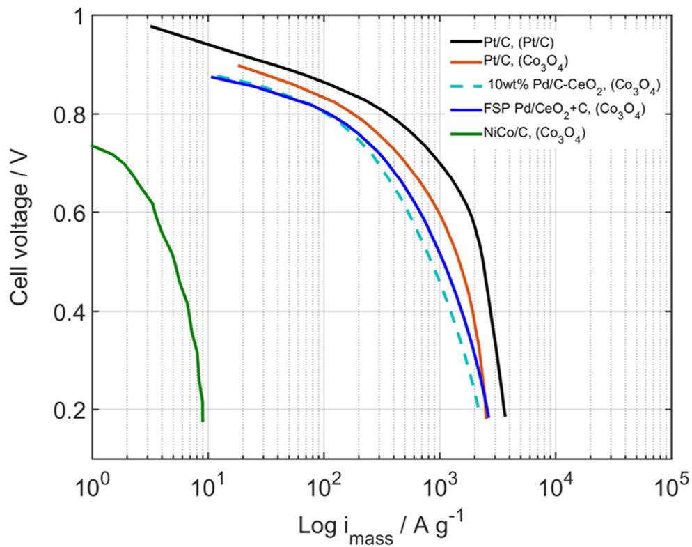
**Figure S7.** AEMFC polarisation curves normalised to anode catalyst mass (cathodes are denoted within parenthesis in the legend). Measurements taken at 70 °C, H<sub>2</sub> and O<sub>2</sub> on anode and cathode, using 1.0 and 0.5 slpm, respectively. Gas dew point 68 and 73 °C for the anode and cathode, respectively.
