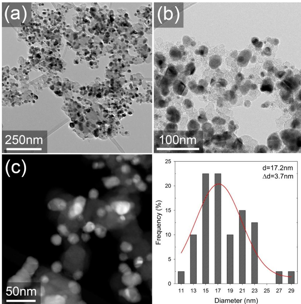
Figure S3. (a,b) Bright Field and (c) Dark Field images of annealed NiCo/C- nanoparticles at various magnifications. (d) Size histogram of the annealed particles from image analysis.
