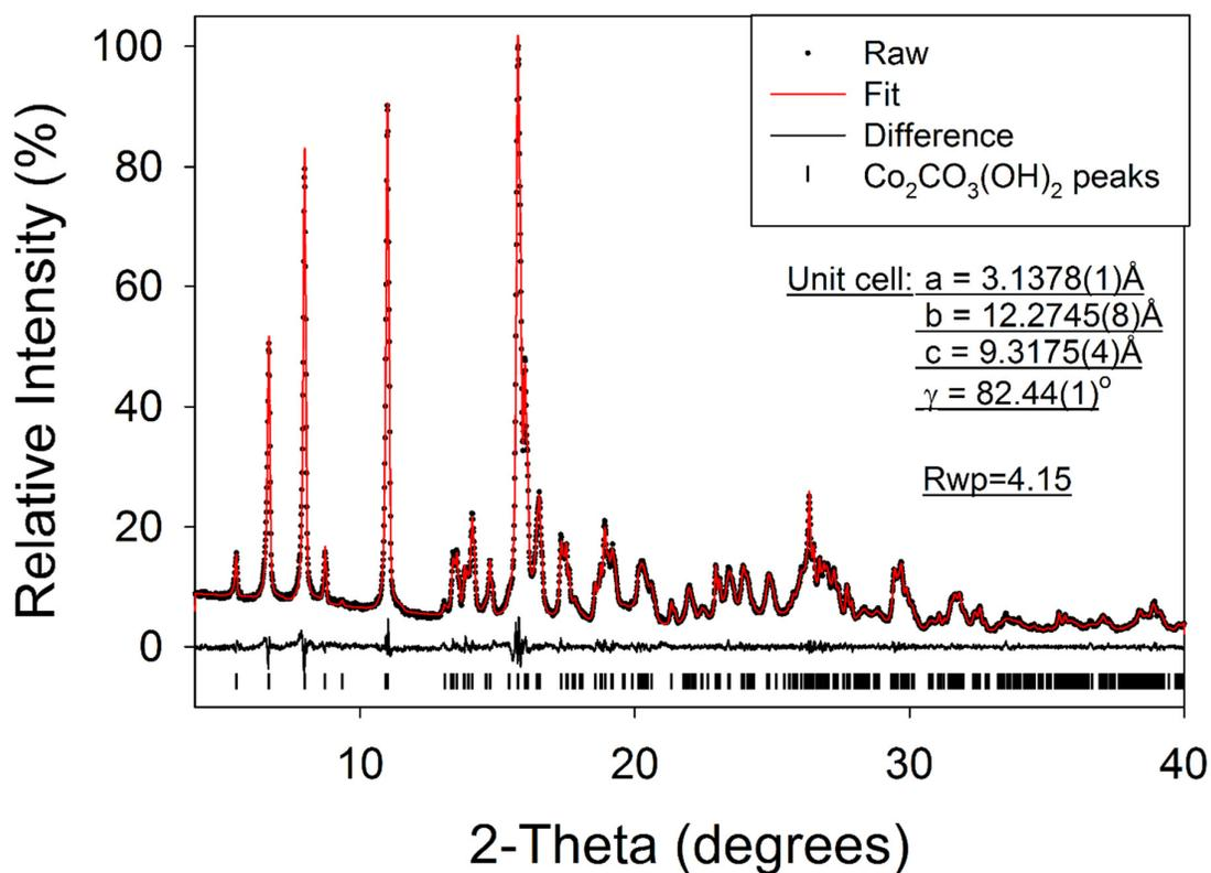
**Figure S1.** Fitted x-ray diffractogram for the Co<sub>2</sub>(CO<sub>3</sub>)OH<sub>2</sub> intermediate phase. Data were collected in capillary transmission mode using a Mo-K<sub>α</sub> source, and were fitted using a structureless "Pawley" type approach. Space group and unit cell values were taken from González-López et. al. (J González-López, J.K. Cockroft, A. Fernández-González, A. Jiménez, R. Grau-Crespo. *Acta Cryst.*, **2017**, B73, 868-873).
