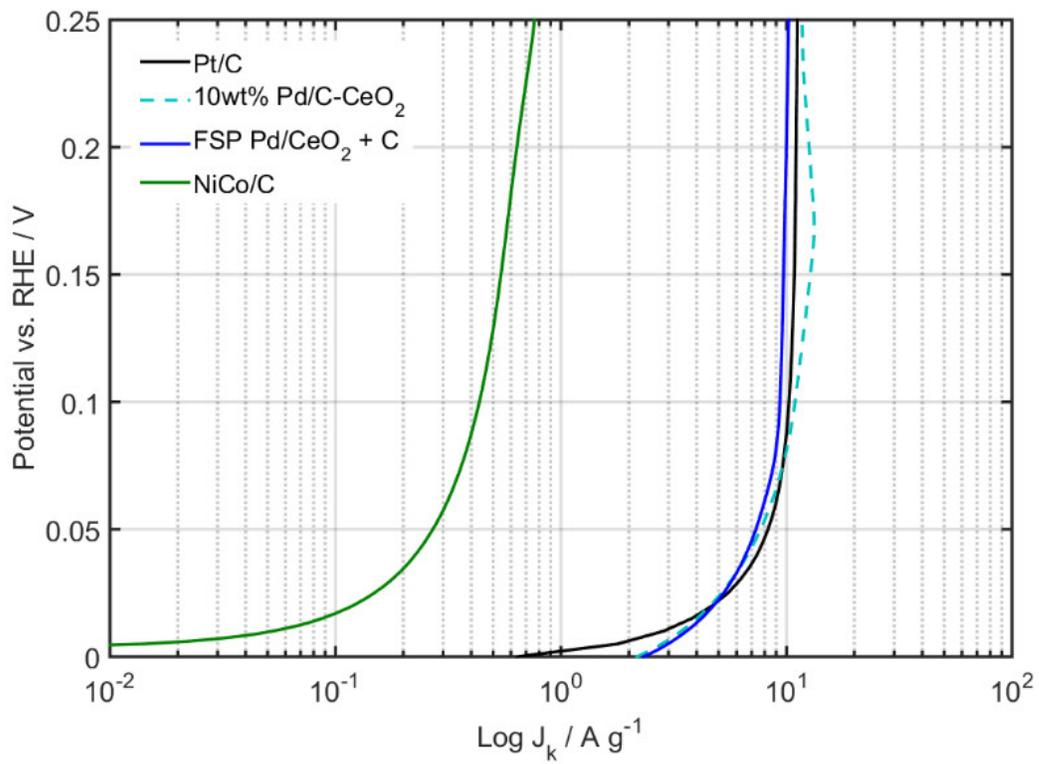
**Figure S6.** Mass activities of HOR catalysts in RDE. H<sub>2</sub>- saturated 0.1 M KOH. Scan rate: 5 mV/s, the catalyst loading was 500  $\mu$ g based on Ni and for the PGM catalysts 50  $\mu$ g, rotating speed 1600 rpm.
