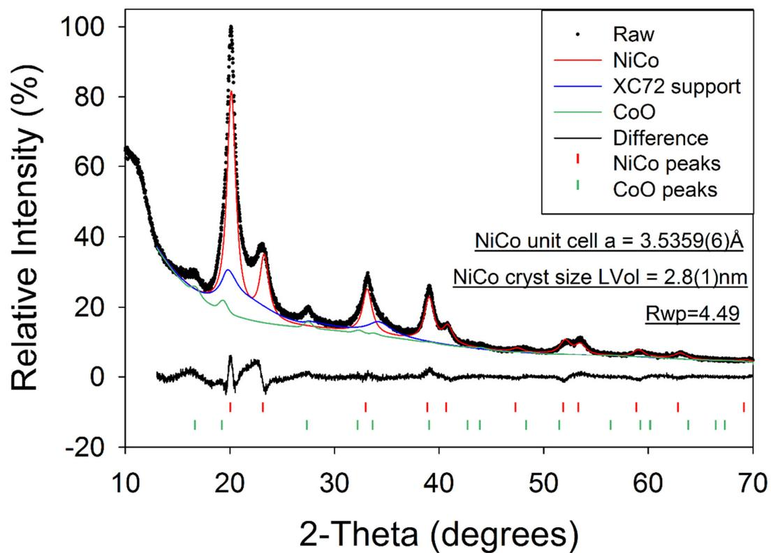
**Figure S2.** Fitted x-ray diffraction pattern for NiCo/C, as-prepared. Data were collected in capillary transmission mode using a Mo- $K\alpha$  source, and modelled using a Rietveld type approach. The background contribution from XC72 carbon was modelled from a separate scan.
