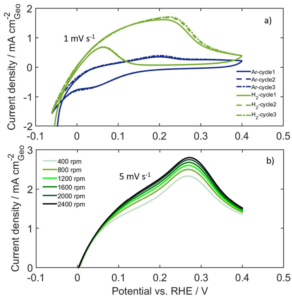
**Figure S5.** (a) Cyclic voltammograms of NiCo/C in both Ar-saturated and H<sub>2</sub>-saturated 0.1M KOH, Scan rate: 1 mV/s and rotating speed 1600 rpm. (b) LSVs of NiCo/C in H<sub>2</sub>- saturated 0.1 M KOH. Scan rate: 5 mV/s at different rotating speeds. The catalyst loading was 500  $\mu$ g metal.
