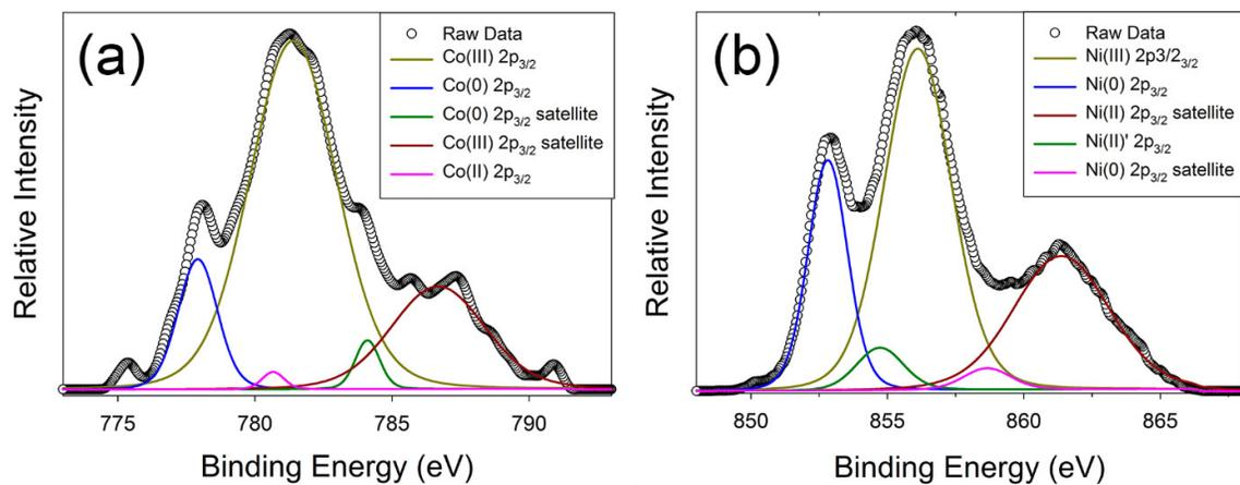
Figure S4. Fitted XPS spectra of (a) Co<sub>2p</sub> and (b) Ni<sub>2p</sub> regions.
