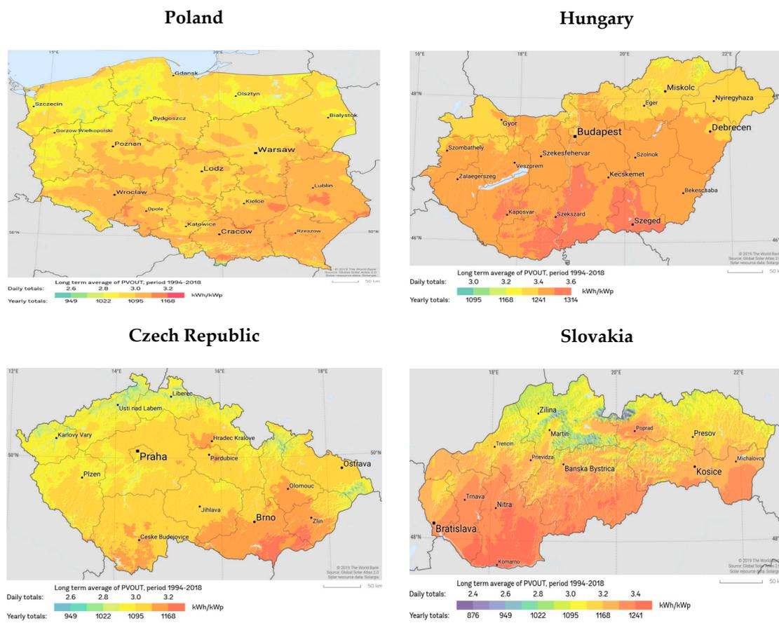
Figure 1. The photovoltaic power potentials of the V4 countries [67].
