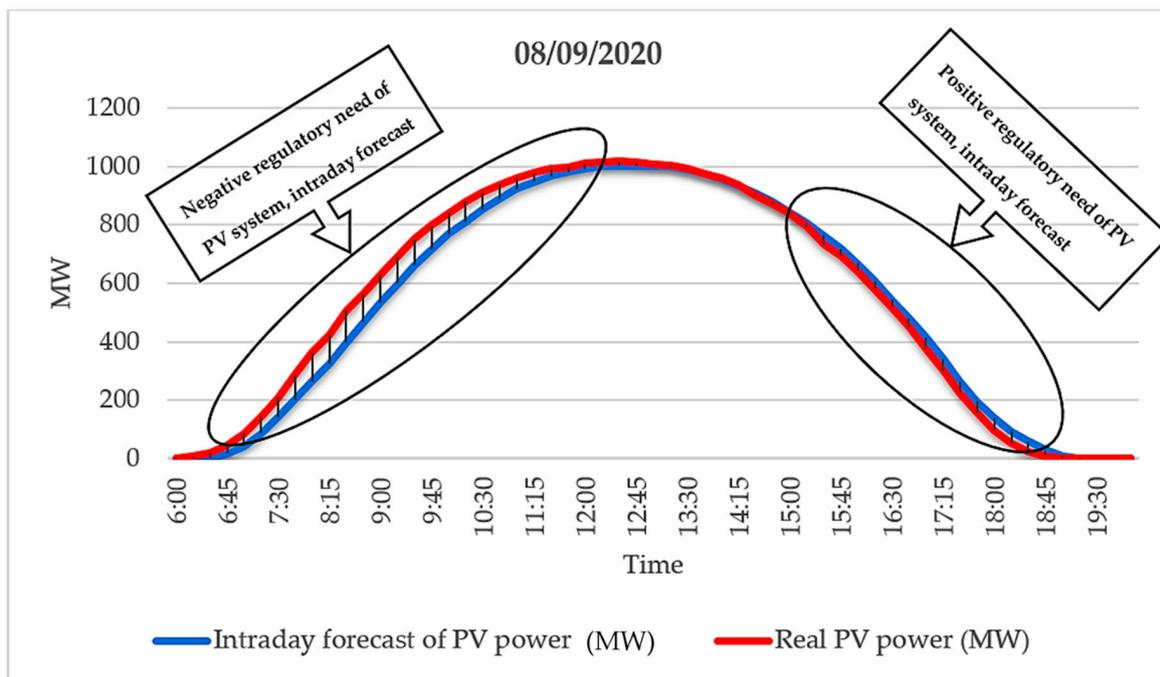
**Figure 2.** A Hungarian example to illustrate the deviation of real PV power generation and intraday forecast data in the case of a monitored 1196 MWp PV system, 8 September 2020 [81].
