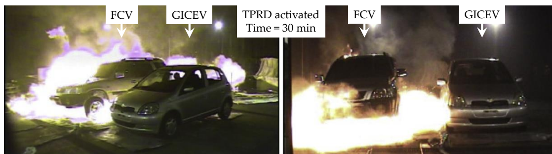
Figure 6. A fireball ignited by a controlled H_2 release managed by a TPRD—Two different views of the front of the vehicles (left a default FCV, and right a classic and undamaged gasoline vehicle (GICEV)) [76].
