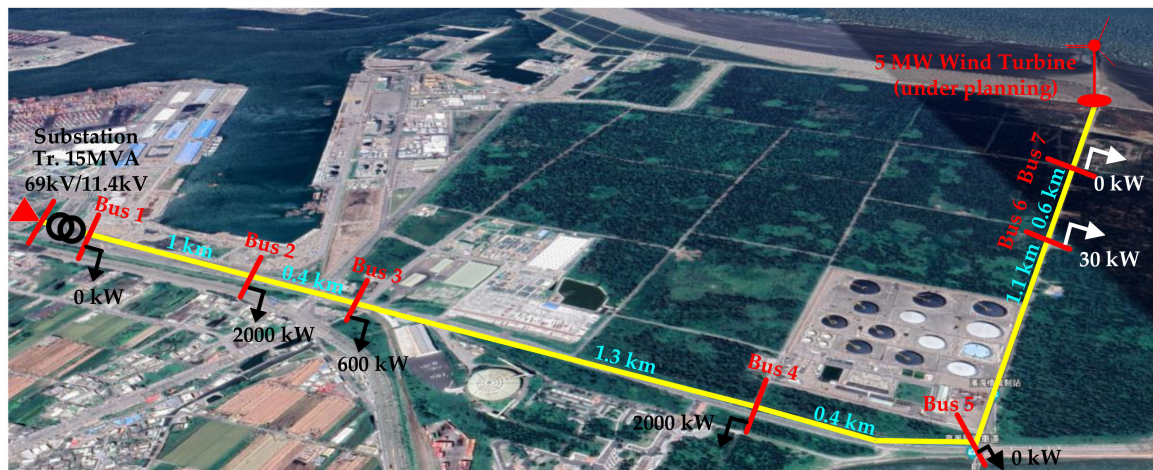
Figure 5. 7 bus testing distribution feeder for PV hosting capacity (PVHC) analysis.
