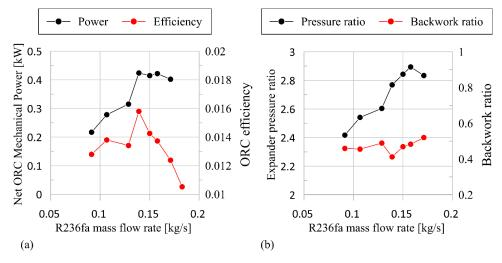
**Figure 10.** (a) Net power produced by ORC and efficiency; and (b) expander pressure ratio and backwork ratio.
