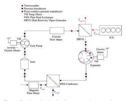
Figure 1. Experimental test bench and measurement instruments layout.
