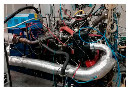
**Figure 3.** IVECO F1C 3-L supercharged diesel internal combustion engine.
