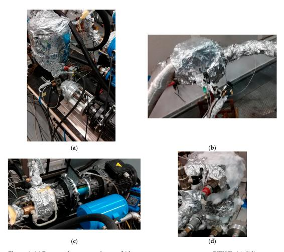
**Figure 4.** (a) Pump and upstream plenum; (b) heat recovery vapour generator (HRVG); (c) sliding vane rotary expander (SVRE); (d) plate heat exchanger (PHX) condenser.
