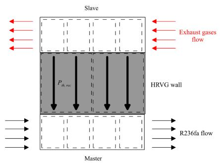
Figure 6. Modeling approach for the HRVG based on the master and slave parameterization.
