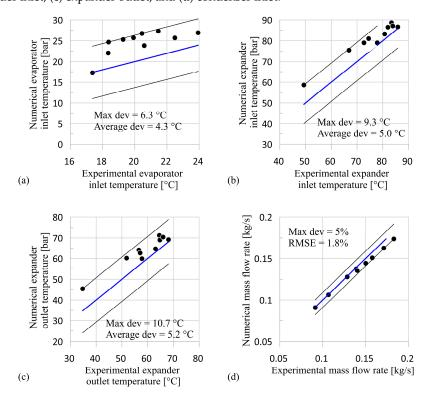
**Figure 8.** Comparison between the experimental and predicted (a) temperature at evaporator inlet; (b) temperature at expander inlet; (c) temperature at expander outlet; and (d) WF mass flow rate.
