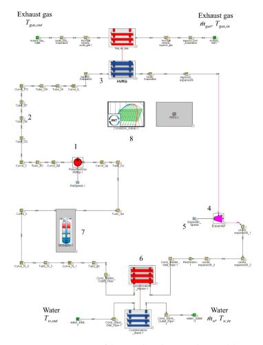
Figure 5. Diagram of the ORC-based power plant model.
