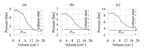
**Figure 11.** SVRE experimental indicated cycle: (a) overexpansion; (b) nominal expansion; and (c) underexpansion.
