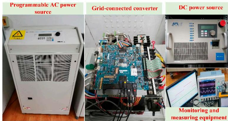
Figure 10. Experimental setup for a three-phase converter.
