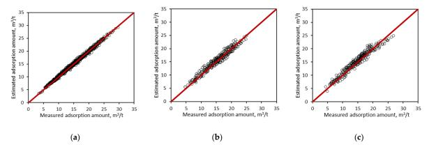
**Figure 6.** Cross plot of the gradient boosting decision trees (GBDT) estimated versus measured adsorption amount for the (a) training (b) validation; and, (c) testing sets. Open circles are data points; red lines are 45-degree lines.
