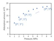
**Figure 3.** An example of the experimentally measured adsorption isotherm represented with discrete equilibrium points.  $P^i$  and  $Y^i$  represent the equilibrium pressure and the corresponding adsorption amount for the ith equilibrium points.
