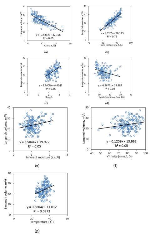
**Figure 4.** Correlation analysis of input features with the adsorption capacity represented with Langmuir volume. (a) ash (a.r.); (b) fixed carbon (d.a.f.); (c) vitrinite reflectance; (d) inherent moisture (a.r.); (e) equilibrium moisture; (f) vitrinite (m.m.f) and (g) temperature.
