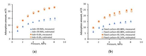
**Figure 7.** Comparison of the estimated with measured adsorption isotherms for samples with (a) ash contents of 9.6% and 39.96%, respectively, and (b) fixed carbon contents of 83.88% and 91.54%, respectively.
