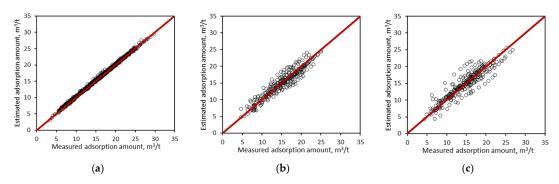
**Figure 8.** Cross plot of the BP-ANN estimated versus measured adsorption amounts for the (a) training, (b) validation, and (c) testing sets. Open circles are data points; red lines are 45-degree lines.
