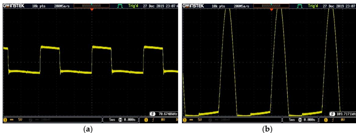
**Figure 16.** Measured waveform using oscilloscope: (a) the radio frequency power supply chip waveform; (b) operating frequency waveform.
