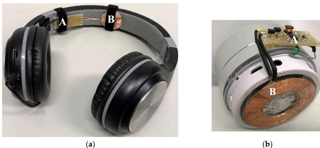
**Figure 19.** The developed wireless receiver module installation: (a) on the wireless headphone (part A is receiver module and part B is receiver coil); (b) on wireless portable audio speaker (part A is receiver module and part B is receiver coil).
