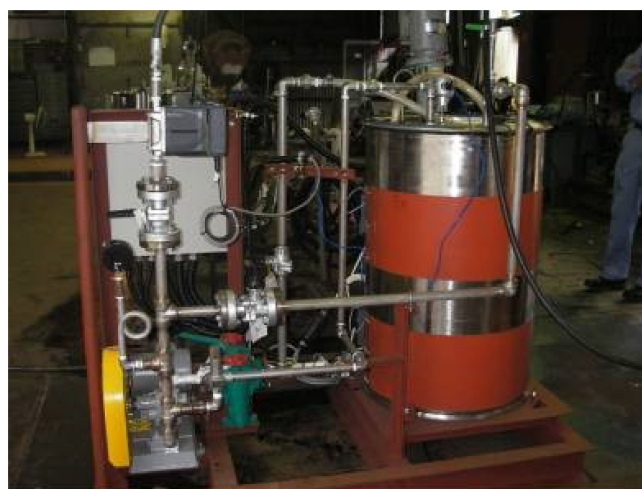
Figure 5. Bio-oil and A-fuel oil co-combustion test equipment.
