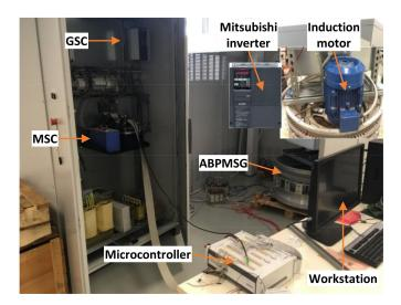
Figure 10. Experimental test rig.
