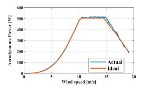
Figure 17. Actual and ideal aerodynamic power curves depending on wind speed.
