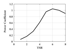
Figure 3. DHAWT characteristic curve.
