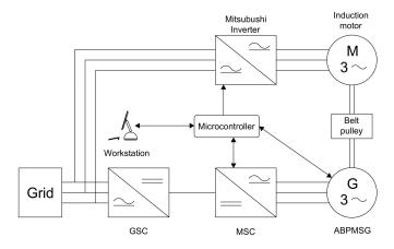
Figure 11. The test rig's logical scheme.
