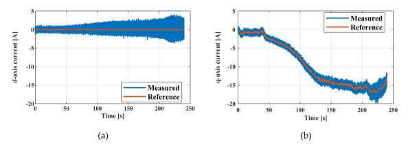
**Figure 15.** Comparison between reference and measured currents: (a) *d*-axis current; (b) *q*-axis current.
