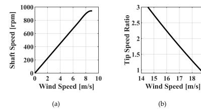
Figure 6. Look-up tables (LUT)s of the control algorithm. (a) Shaft speed reference during MPPT control. (b) Tip-speed ratio (TSR), during constant torque control (CTC).
