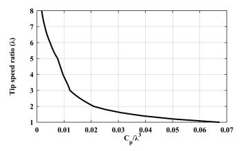
**Figure 9.**  $\frac{C_p}{\lambda^3} - \lambda$  characteristic.
