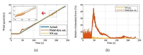
**Figure 12.** Wind speed: (a) actual and estimated wind speed pattern; (b) relative (percentage) estimation errors.
