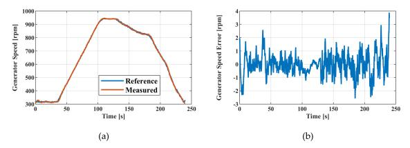
**Figure 14.** ABPMSG rotor speed: (a) speed reference and measured rotor speed; (b) absolute speed tracking error.
