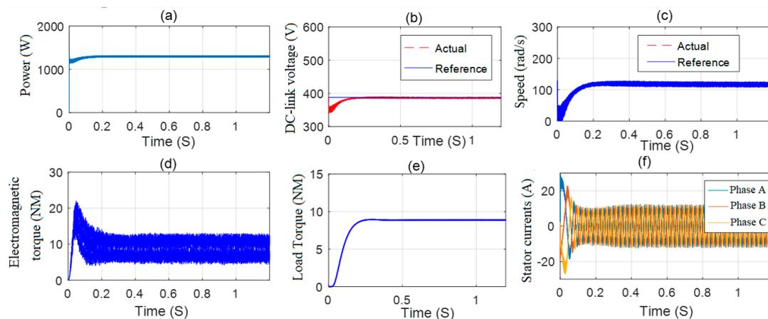
Figure 9. Performance of SPVWPS under partial shading condition using COA algorithm tuned PI controller of the DC link voltage and rotor speed. (a) power; (b) DC voltage; (c) speed; (d) electromagnetic torque; (e) load torque and (f) stator currents.
