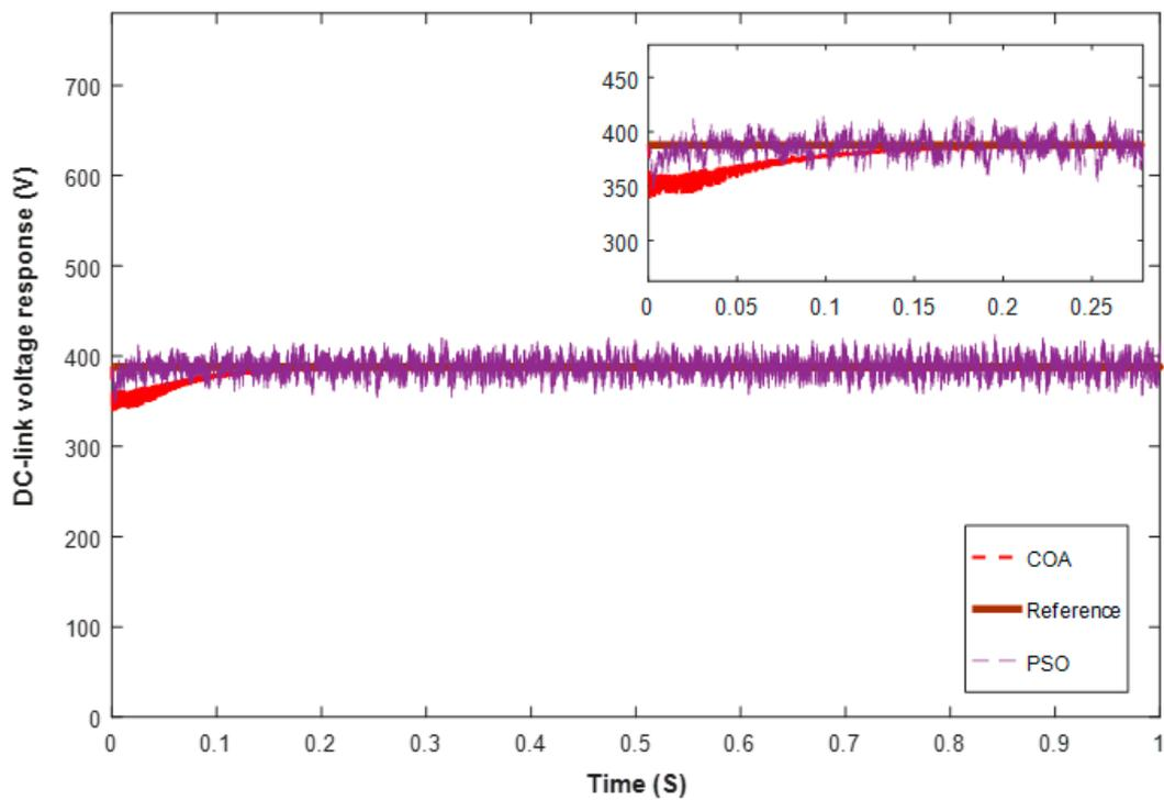
Figure 8. DC-link voltage responses using particle-swarm optimization (PSO) and COA.
